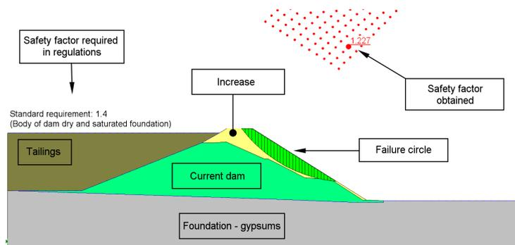
Fig. 14 Safety factor of the failure circle
