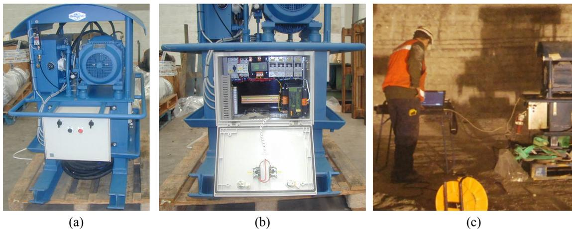
Fig. 3 (a) Hydraulic power unit; (b) Electrical switchboard and data capture system; (c) Connection to computer
