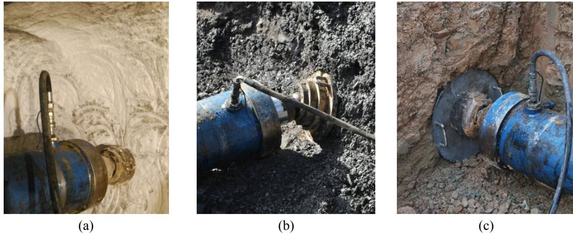
Fig. 2 Applying pressure to the tested soil using different sizes of plates
