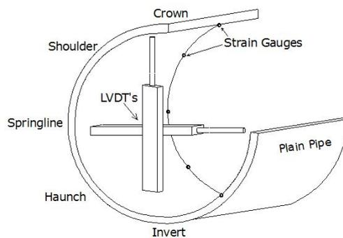
Fig. 3 Section through lined-plain pipe
