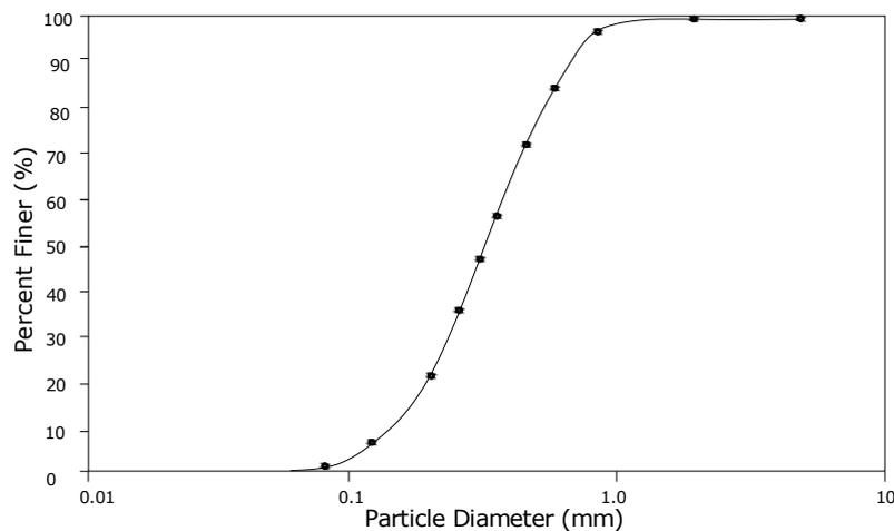
Fig. 4 Sieve analysis of sand particles
