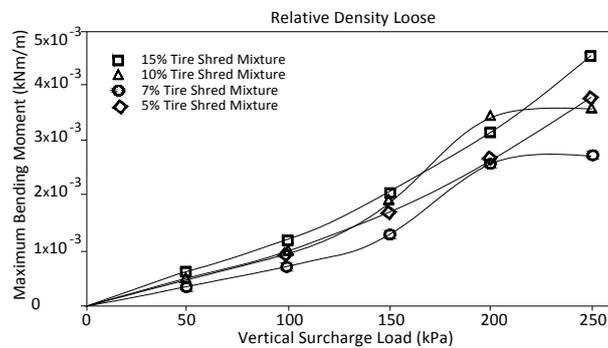
Fig. 13 Maximum bending moment at loose backfill condition
