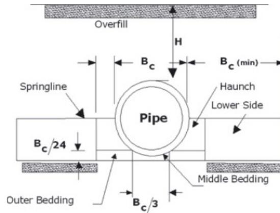
Fig. 1 A Conventional standard trench section (ASTM D 2321)
