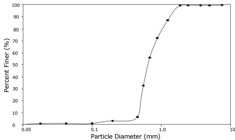
Fig. 6 Sieve analysis of tire shreds
