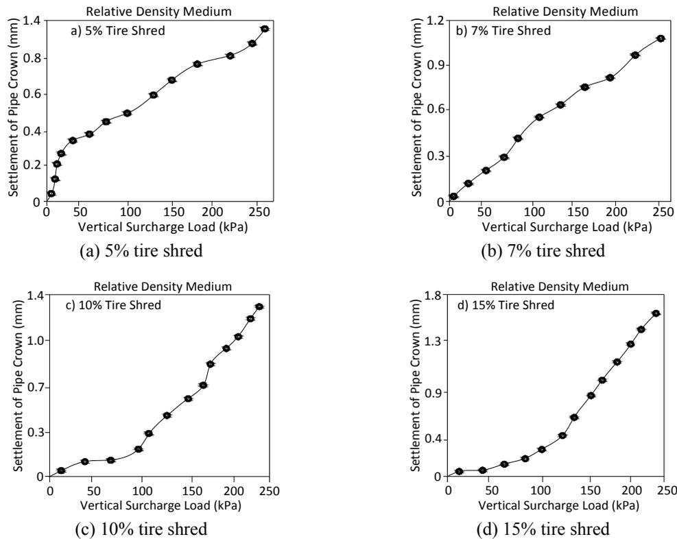
Fig. 11 Vertical deflection of pipe crown in medium backfill condition
