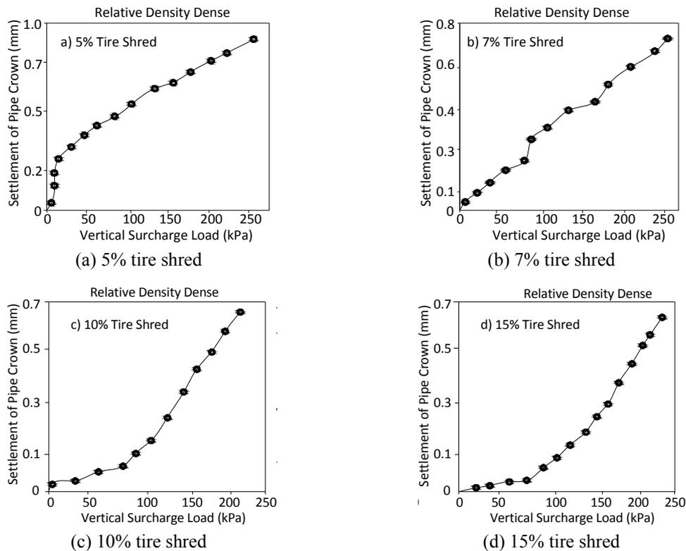
Fig. 12 Vertical deflection of pipe crown in dense backfill condition
