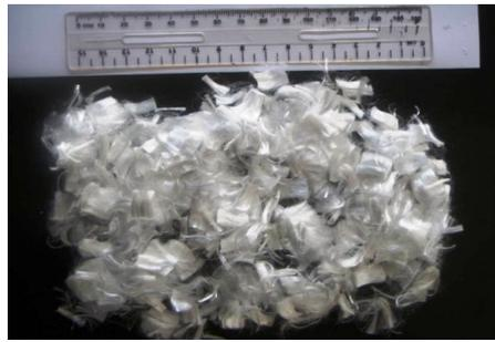
Fig. 1 Polypropylene fibres used in the study
