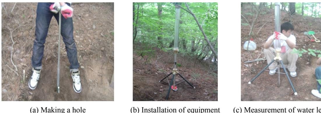
Fig. 2 Process of Guelph permeameter experiment
