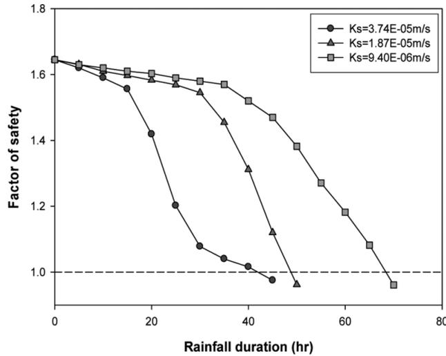
Fig. 1 FS (Factor of safety) of slope versus soil hydraulic conductivity (Ministry of Science, ICT and Future Planning of Korea 2013)
