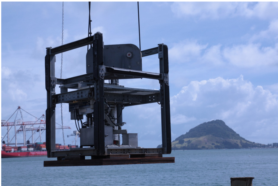
Fig. 2 The Geotechnical offshore seabed tool during deployment in Stella Passage, Tauranga Harbor
