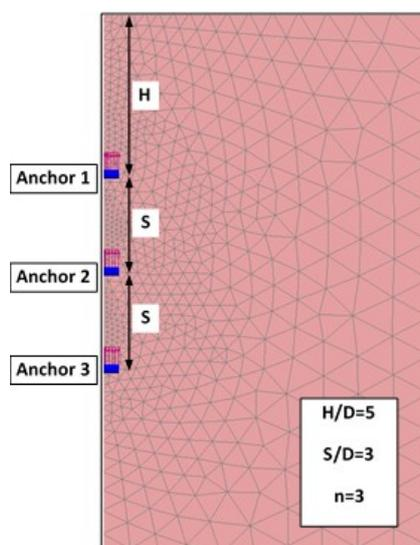
Fig. 4 Typical mesh configurations in the FE Analyses
