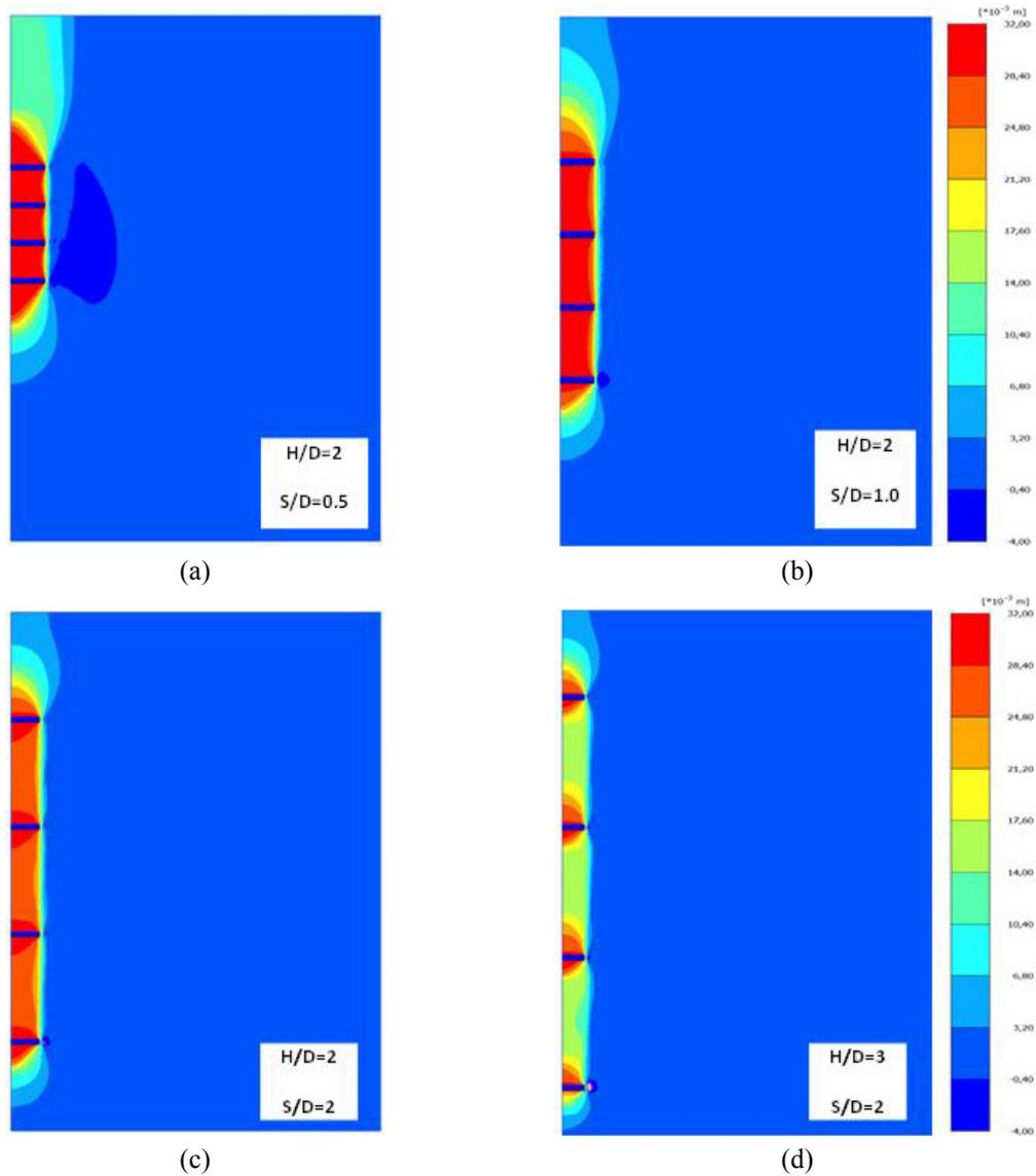
Fig. 9 Displacement contours illustrating transition from shallow global to shallow individual plate failure mode ( $n = 4$ )
