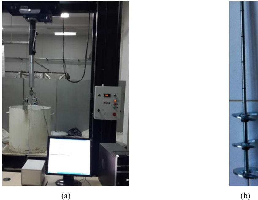
Fig. 1 Test set-up: (a) overview; (b) helical anchor plate
