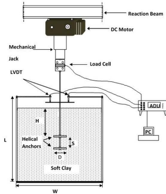
Fig. 2 General layout of apparatus for the model test
