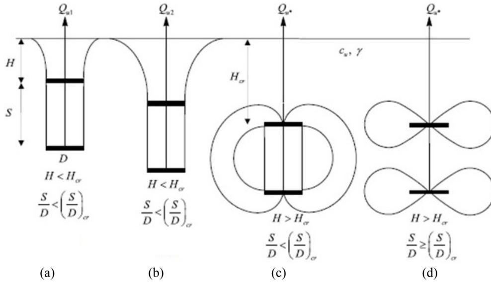
Fig. 6 Shallow and deep anchor behavior: (a) and (b) shallow failure mechanism; (c) global deep failure mechanism; (d) local deep failure mechanism (Merifield 2011)
