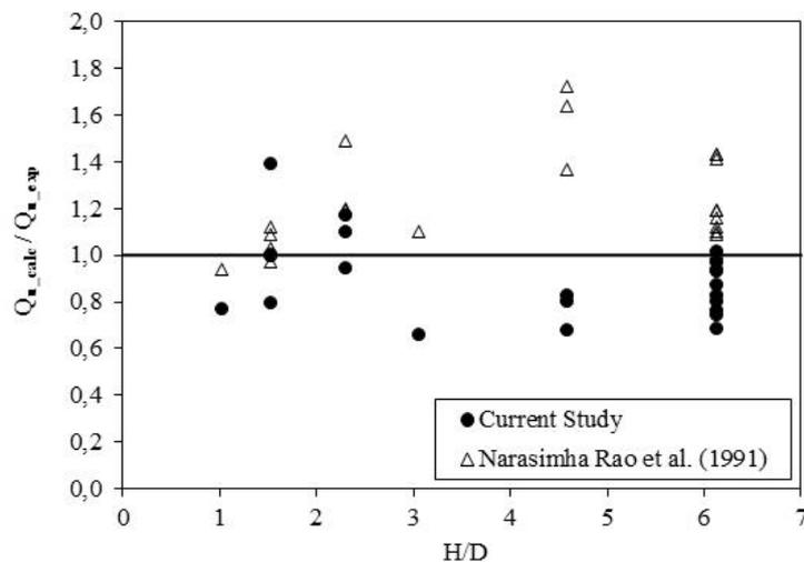
Fig. 11 Comparison between numerical and laboratory results for multihelical plate anchors
