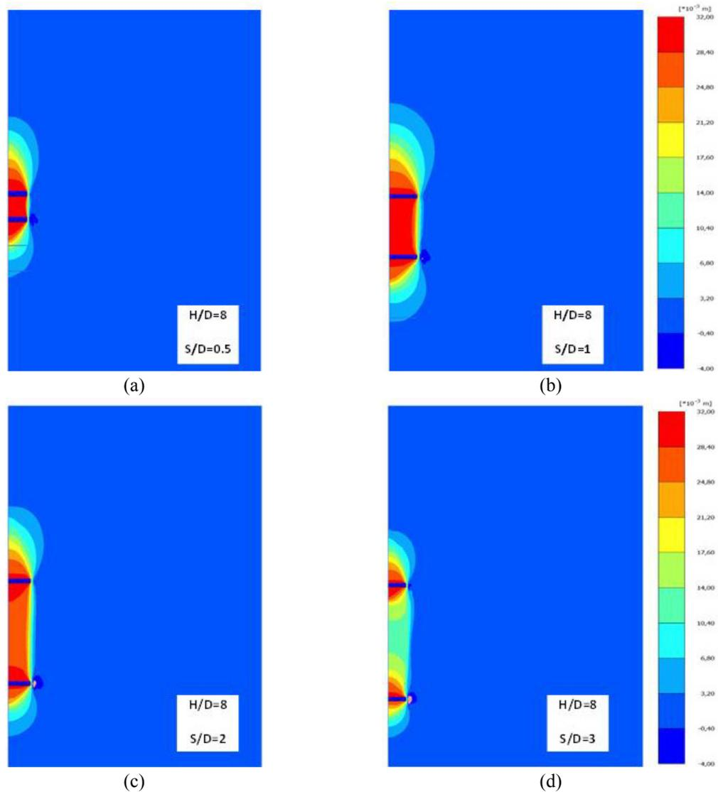
Fig. 10 Displacement contours illustrating transition from deep global to deep individual plate failure mode ( $n = 2$ )
