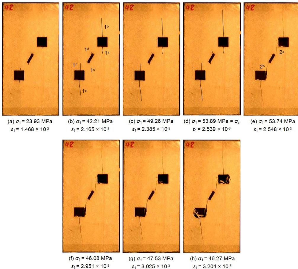
Fig. 14 Crack evolution process of sandstone specimen containing combined flaws ( $\alpha = 60^\circ, \beta = 60^\circ$ ) with the increase of deformation. The denoted letter shown in the figure is corresponding to Fig. 13
