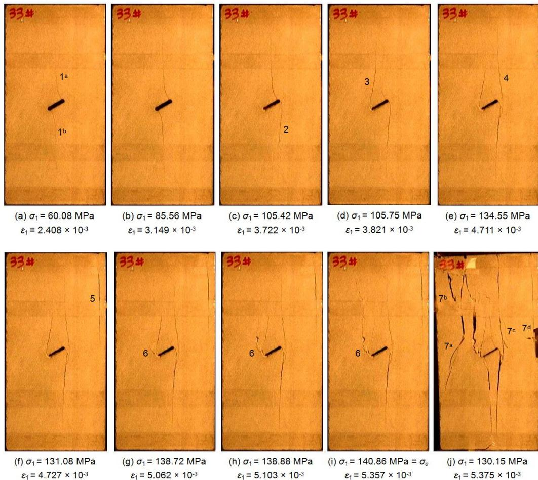
Fig. 7 Crack evolution process of sandstone specimen containing a single fissure ( $\alpha = 30^\circ$ ,  $2a = 15$  mm) with the increase of deformation. The denoted letters shown in the figure are corresponding to Fig. 6
