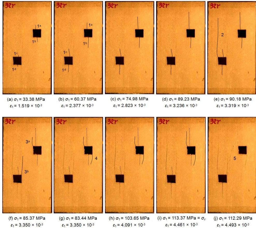
Fig. 9 Crack evolution process of sandstone specimen containing double squares with the increase of deformation. The denoted letters shown in the figure are corresponding to Fig. 8
