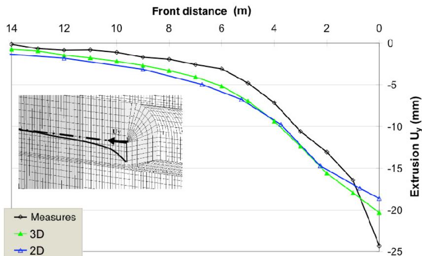
Fig. 10 Measured deformations at the tunnel face and comparison with the corresponding curves of the 2D and 3D models
