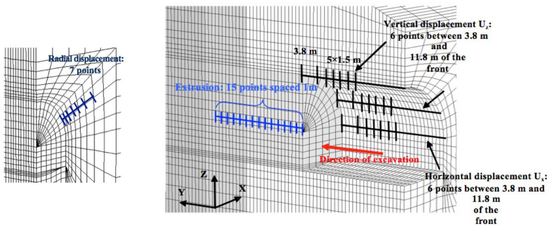
Fig. 9 Measurements considered in the inverse analysis process of section M6 with the 3D model
