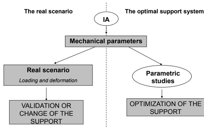
Fig. 2 Scheme of how to use inverse analysis in the scope of the developed methodology
