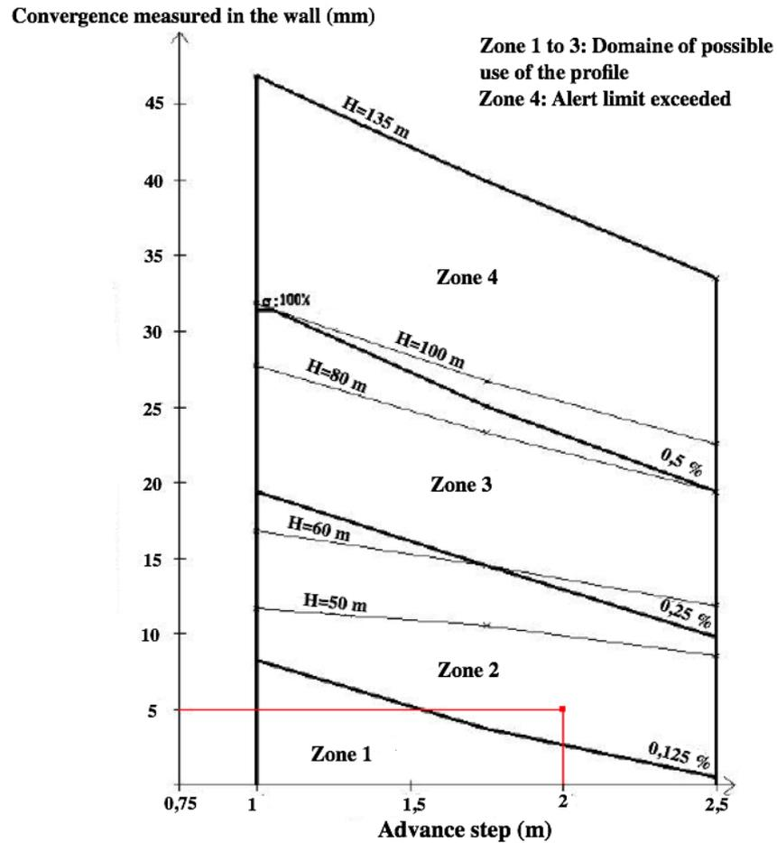
Fig. 7 Use of the graphic to evaluate the scenario for section M4
