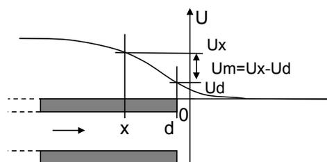
Fig. 3 Scheme for the  $U_m$  calculation (ordinates of the graphics)
