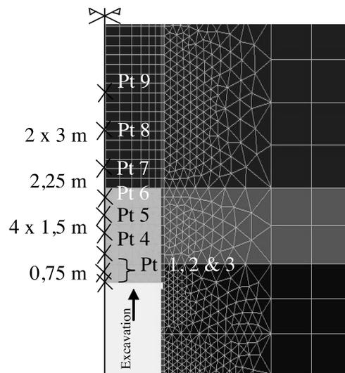
Fig. 8 Location of the measurement points considered in the inverse analysis process of section M6 with the 2D model
