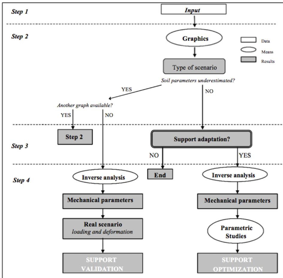
Fig. 1 Proposed methodology for the support adaptation
