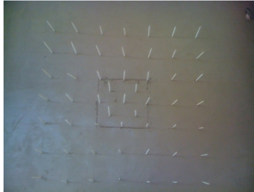
Fig. 6 Spacing of grouted points in the soil
