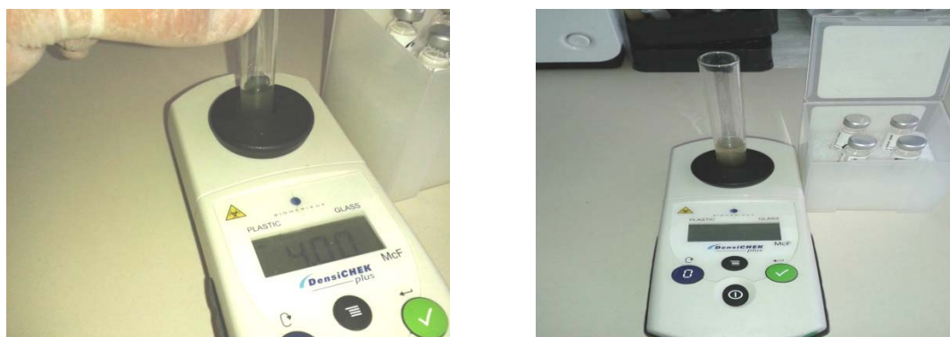
Fig. 1 DensiCHEK Plus instrument used to measure the optical density of a microorganism suspension
