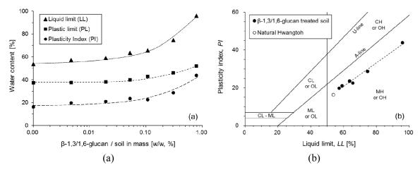
Fig. 3 Atterberg limits of  $\beta$ -1,3/1,6-glucan (BG) treated Korean residual soil: (a) *LL*, *PL*, and *PI*; (b) Plasticity chart
