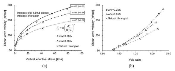
Fig. 6 Shear wave velocity of  $\beta$ -1,3/1,6-glucan (BG) content treated Korean residual soil: (a) with vertical effective stress; and (b) with void ratio
