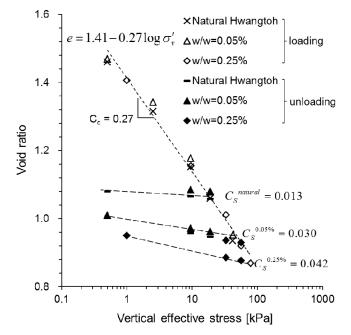
Fig. 5 Void ratio – vertical effective stress relationship of  $\beta$ -1,3/1,6-glucan (BG) treated Korean residual soil
