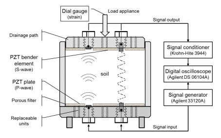
Fig. 1 Schematic diagram of instrumented consolidation testing device
