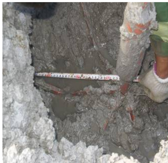
Fig. 8 Photograph of an excavated US anchor in the field
