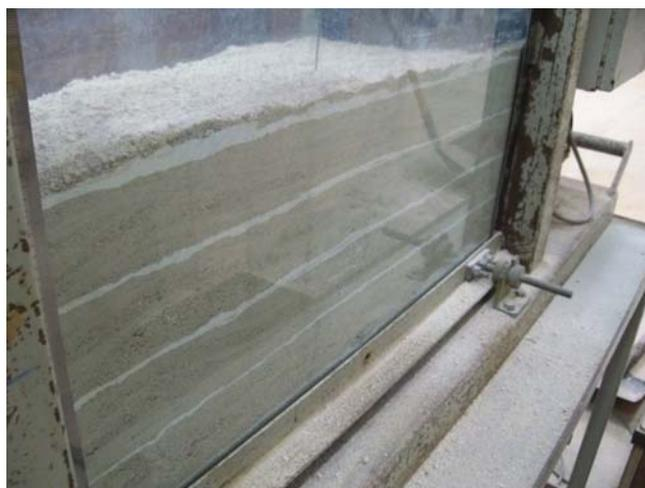
Fig. 11 Initial state of sand before commencement of uplift in loose sand
