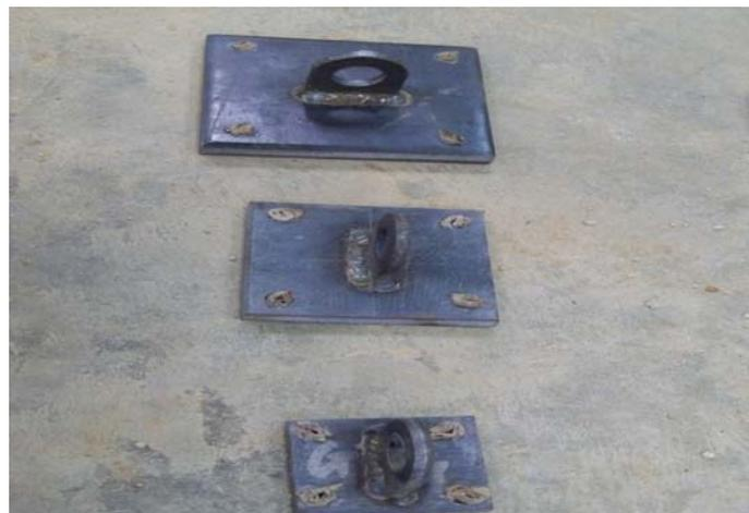
Fig. 4 Symmetrical square anchor plates
