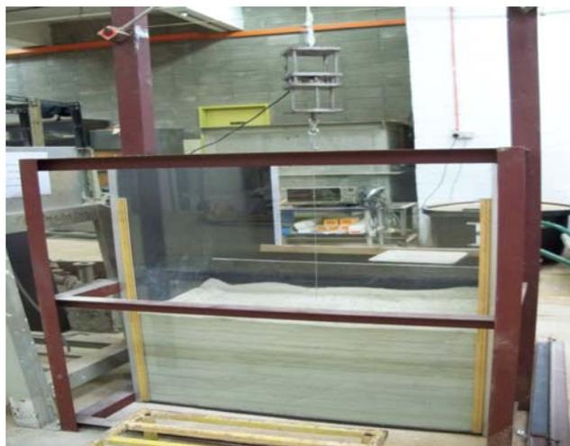
Fig. 5 The setup of the uplift test
