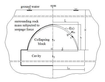
Fig. 1 Collapsing patterns for rectangular cavity subjected to seepage forces
