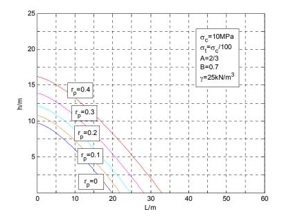
Fig. 3 Shape of collapsing block with respect to different pore pressure coefficients
