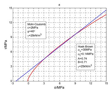
(a) Equivalence relationship between Hoek-Brown failure criterion and Mohr-Coulomb one
