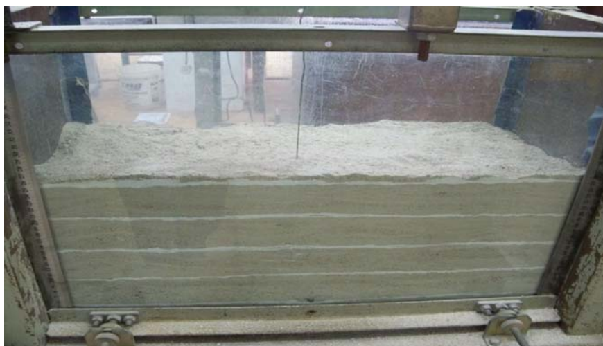
Fig. 13 Initial state of sand before commencement of uplift in loose sand
