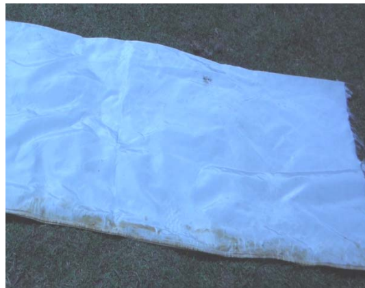
Fig. 3 Geotextile used to reinforce the sand column
