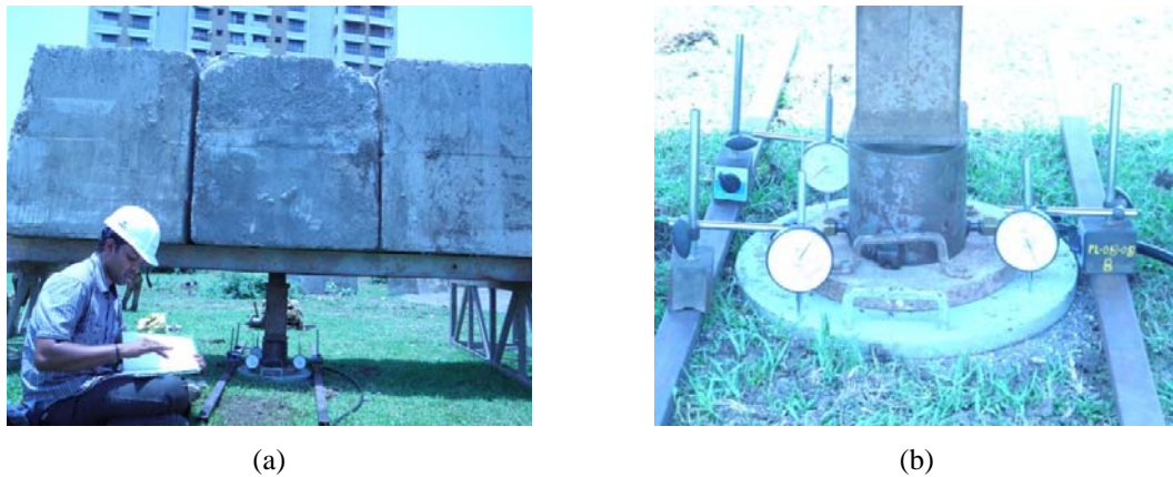
Fig. 6 Photograph of one of the loading tests: (a) General view; (b) Close view of sand column top
