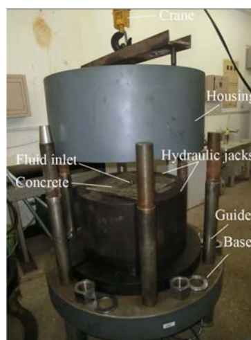
Fig. 1 400^3 \text{ mm}^3 true tri-axial hydraulic fracturing test equipment
