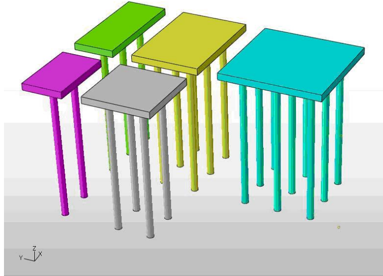
Fig. 1 Three dimensional view of the piled raft configurations adopted in the finite element study
