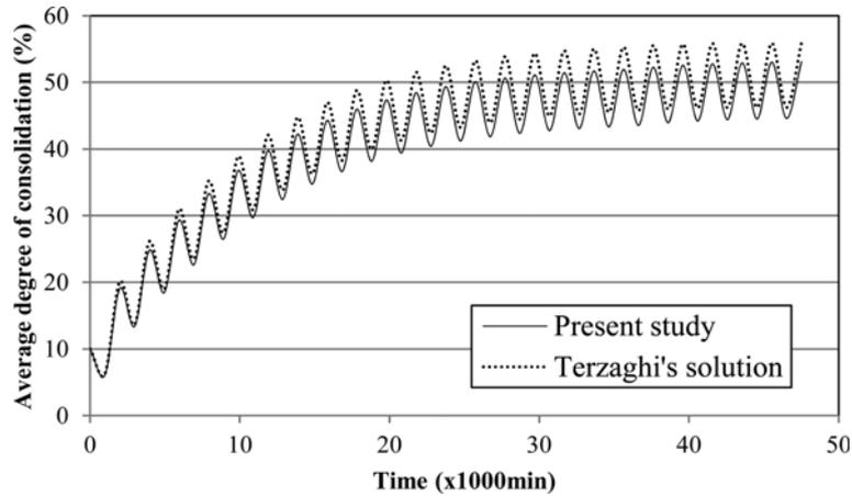
Fig. 3 Variations in the average degree of consolidation under cyclic loading
