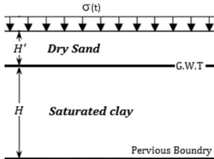
Fig. 1 A saturated clay layer subjected to cyclic loading
