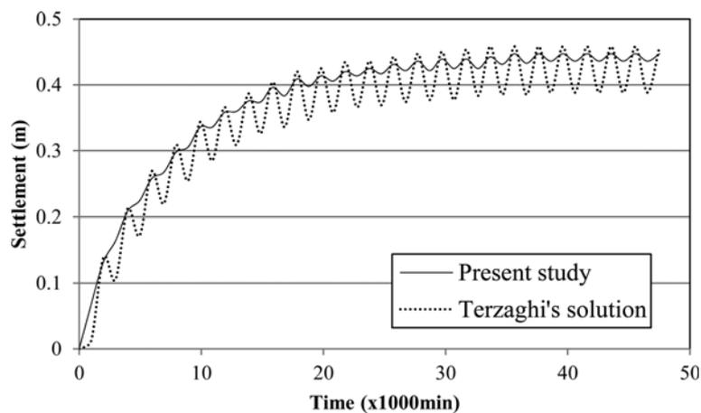
Fig. 4 Variations in the settlement under cyclic loading
