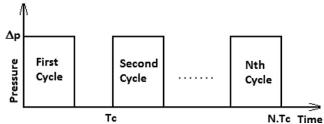
Fig. 2 The scheme of the applied rectangular cyclic loading
