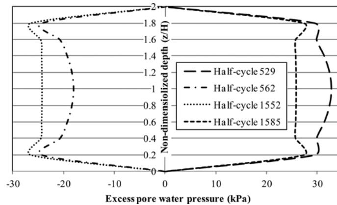
Fig. 5 The excess pore water pressure distribution under cyclic loading
