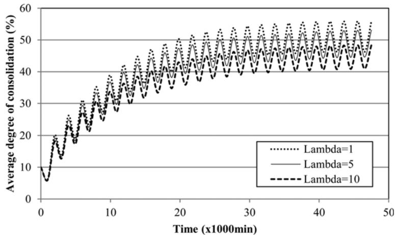
Fig. 6 Effect of clay nonlinearity on the average degree of consolidation
