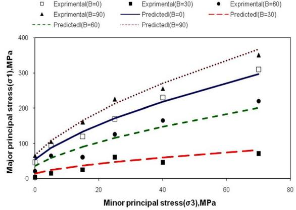
Fig. 20 Variation of strength in model rock (type 10E developed in this study) vs. confining pressure for given angle of plane of weakness ( $\beta$ )
