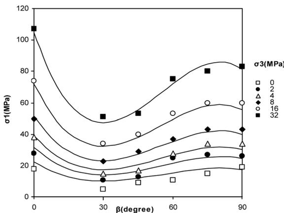
Fig. 17 Strength anisotropy observed in model rock (current study) and prediction by Eq. (18)
