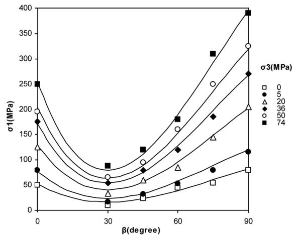
Fig. 18 Strength anisotropy observed in model rock (current study) and prediction by Eq. (18)
