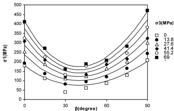
Fig. 11 Strength anisotropy observed in Slate of Penrhyn (Attewell and Sanford 1974) and prediction by Eq. (18)
