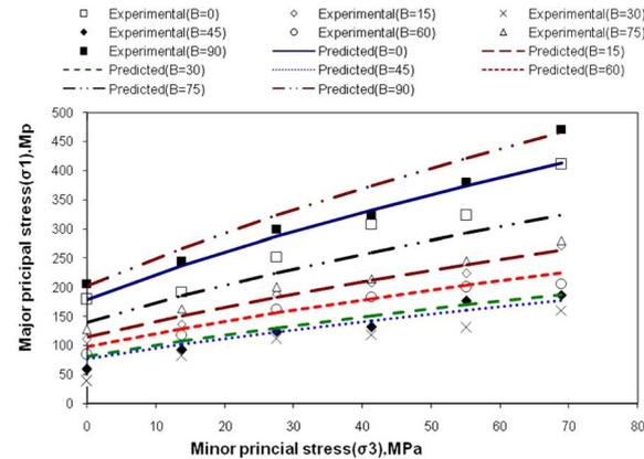
Fig. 21 Variation of strength depicted in principal stress plane ( $\sigma_1 - \sigma_3$ ) for various  $\beta$  observed in Slate of Penrhyn (Attwell and Sanford 1974) and prediction by Eq. (18)
