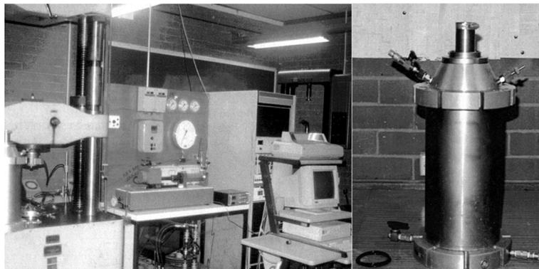
Fig. 6 Triaxial testing apparatus/cell used for the current experiments
