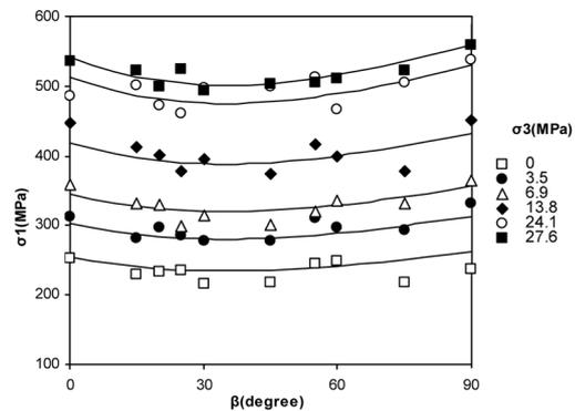
Fig. 12 Strength anisotropy observed in Gneiss (Horino and Ellickson 1970) and prediction by Eq. (18)
