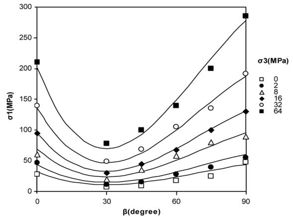
Fig. 16 Strength anisotropy observed in model rock (current study) and prediction by Eq. (18)
