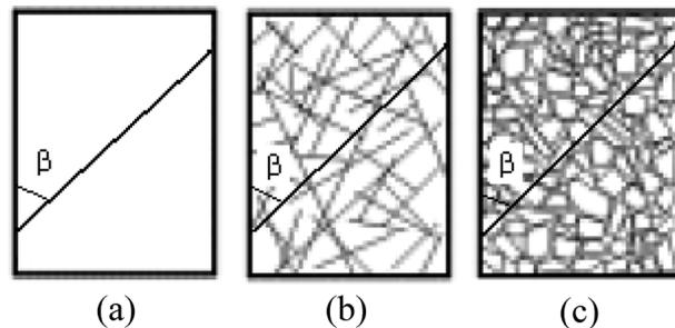
Fig. 4 Samples of anisotropic rock: (a) with intact pieces ( $s = 1$ ); (b) and (c) with crushed pieces ( $0 < s < 1$ )
