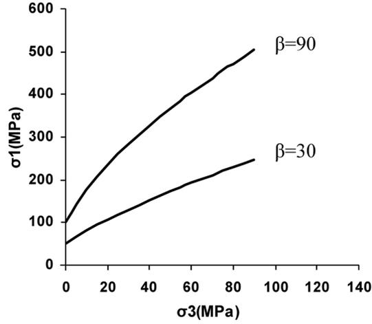
Fig. 5 Strength anisotropy presentation in principal stresses plane for a sample anisotropic rock
