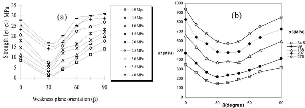
Fig. 10 Strength anisotropy in (a): model rock developed in this study (Bagheripour and Mostyn 1995 and 1996) and (b): Martinsburg slate (Mclamore and Gray 1967)
