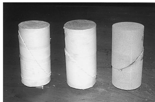
Fig. 9 Some anisotropic model rock samples with single plane of weakness failed in triaxial tests
