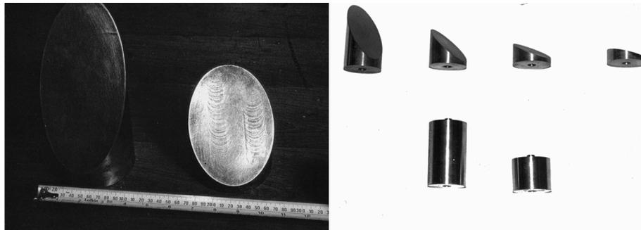
Fig. 7 Typical inclined steel rammers used for development of weakness planes in model rock
