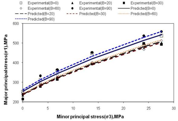
Fig. 24 Variation of strength depicted in principal stress plane ( $\sigma_1 - \sigma_3$ ) for various  $\beta$  observed in Limestone (Horino and Ellickson 1970) and prediction by Eq. (18)
