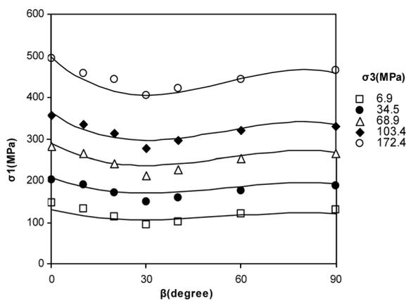
Fig. 13 Strength anisotropy observed in Green River Shale II (McLamore and Gray 1967) and prediction by Eq. (18)
