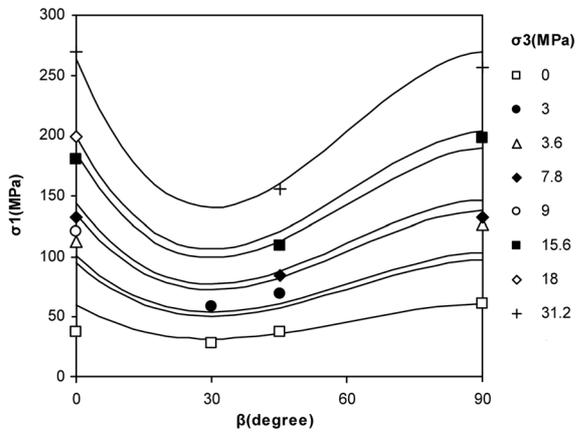
Fig. 15 Strength anisotropy observed in Gneiss (A) (Saroglou and Tsiambaos 2008) and prediction by Eq. (18)
