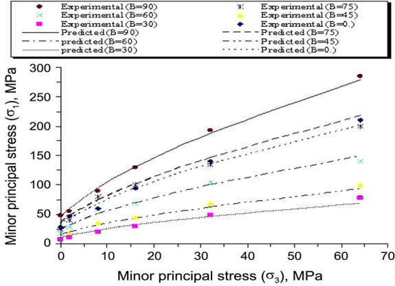
Fig. 19 Variation of strength in model rock (type 10B developed in this study) vs. confining pressure for given angle of plane of weakness ( $\beta$ )
