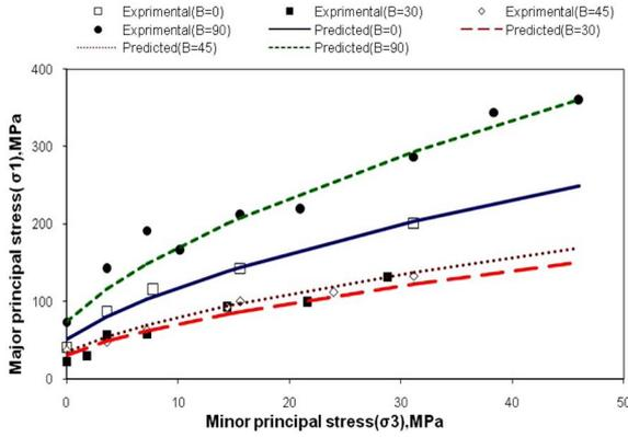
Fig. 23 Variation of strength depicted in principal stress plane ( $\sigma_1 - \sigma_3$ ) for various  $\beta$  observed in Gneiss (B) (Saroglou and Tsiambaos 2008) and prediction by Eq. (18)
