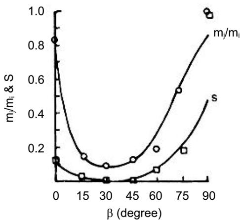
Fig. 3 Variation of  $s$  and  $m_j/m_i$  vs  $\beta$  for anisotropic rock (adopted from Hoek and Brown 1980a)
