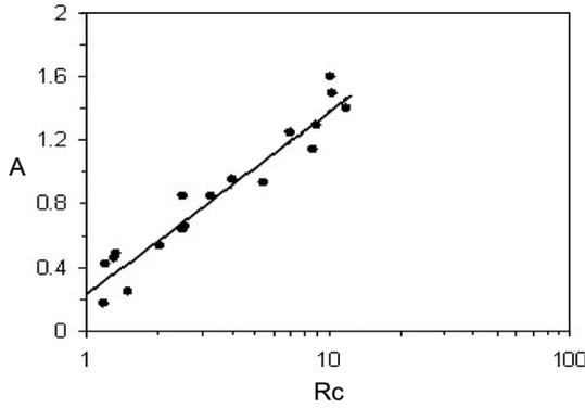
Fig. 25 Variation of parameter  $A$  against anisotropy degree ( $R_C$ )
