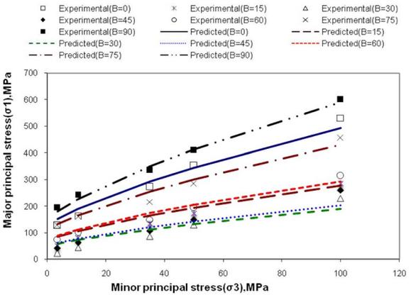
Fig. 22 Variation of strength depicted in principal stress plane ( $\sigma_1 - \sigma_3$ ) for various  $\beta$  observed in Martinsburg Slate (Donath 1964) and prediction by Eq. (18)
