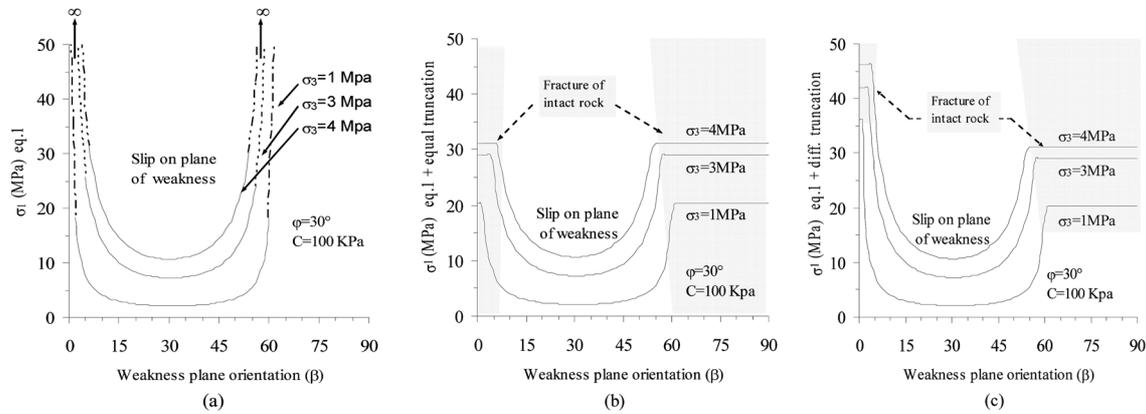
Fig. 2 Graphical presentation of Jaeger (1960) criterion: (a) original criterion with no truncation (b) equal truncation at shoulders (c) differential truncation at shoulders
