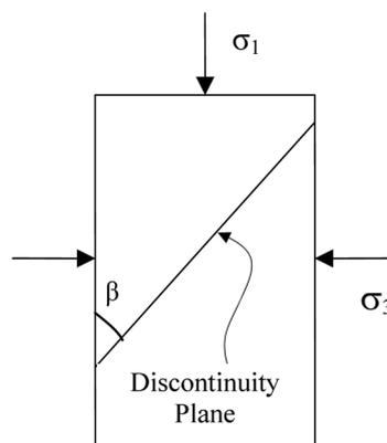
Fig. 1 Anisotropic rock with single plane of discontinuity studied by Jaeger (1960)
