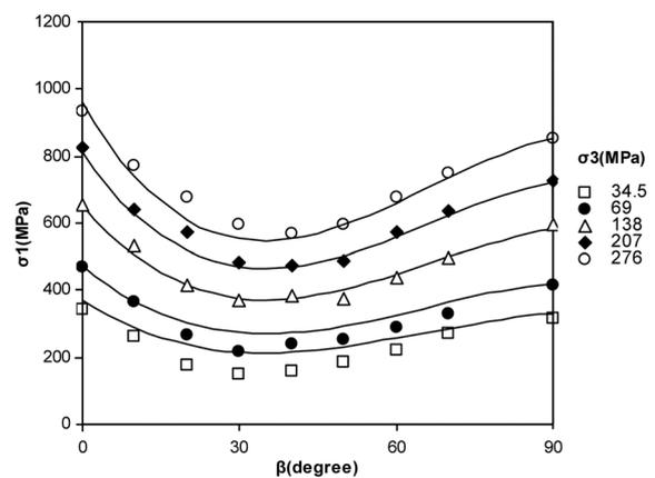
Fig. 14 Strength anisotropy observed in Austin Slate (McLamore and Gray 1967) and prediction by Eq. (18)
