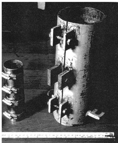
Fig. 8 Split cylinders used to mould and compact the materials for the development of rock and their weakness planes.
