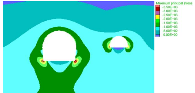
(b) Inter-tunnel distance 1.0D in diverging direction 0°
