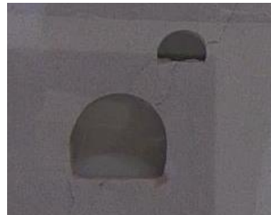
(c) 60° diverging direction at 0.3D inter-tunnel distance
