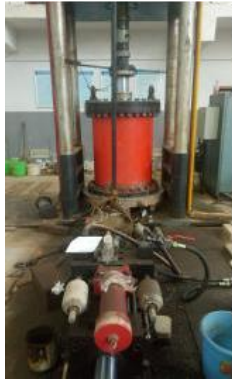
(b) Prepared chamber for confining pressure
