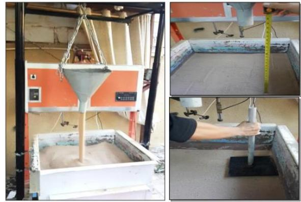
Fig. 5 Raining frame used for controlling sand density
