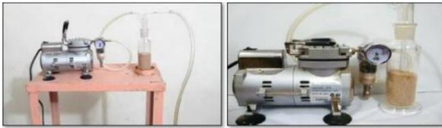
Fig. 7 Soil plug removal system
