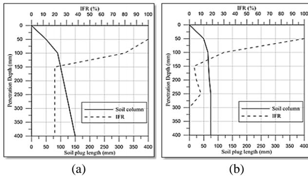
Fig. 1 IFR and soil plug length versus penetration depth for open-ended pile (a-driven, b- pressed) (after Sheghait, 2016)
