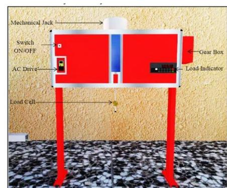
Fig. 3 Steel loading frame and axial loading system.
