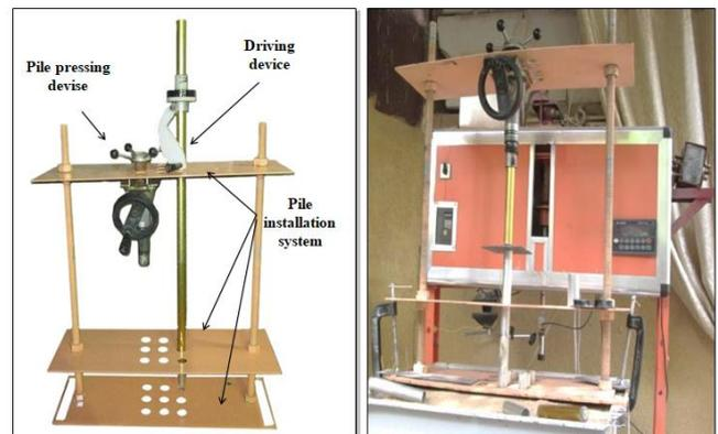
Fig. 6 Pile group system installation
