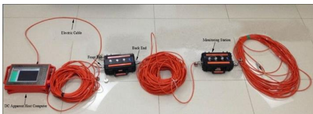
Fig. 4 WBD-type network parallel electrical instrument
