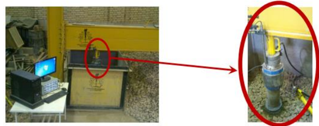
Fig. 5 The assembly of jack, load cell, rigid cylinders and rigid circular plate beneath the strong reaction frame
