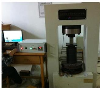
Fig. 8 GAW-2000 rigid testing machine
