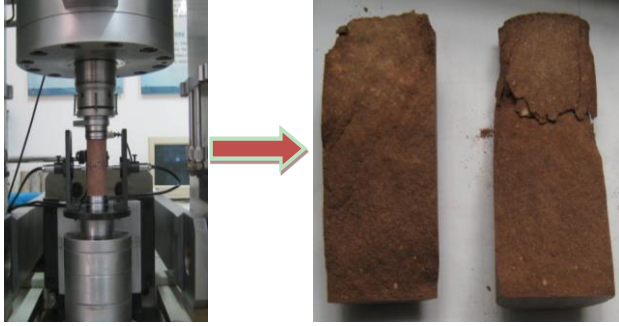
Fig.1 Rock splitting under uniaxial loading
