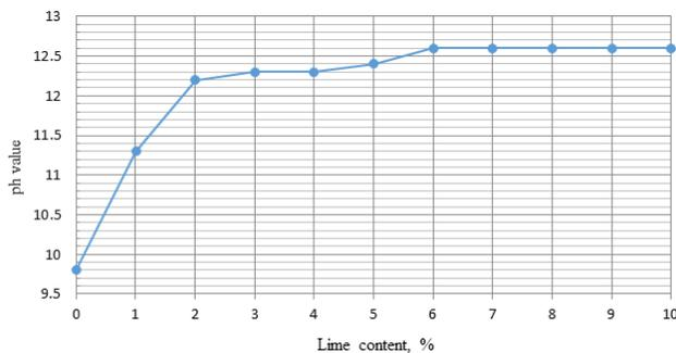
Fig. 6 Effect of various lime content on pH value
