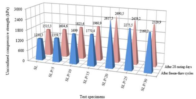
Fig. 12 Comparison of strength before and after freeze-thaw cycles
