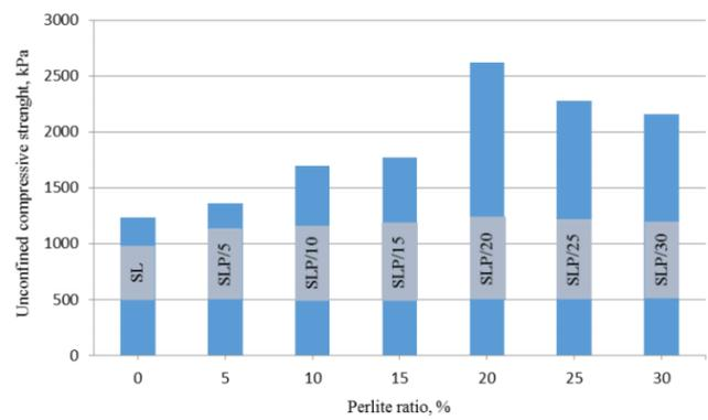
Fig. 11 Unconfined compressive strength after freeze-thaw cycles
