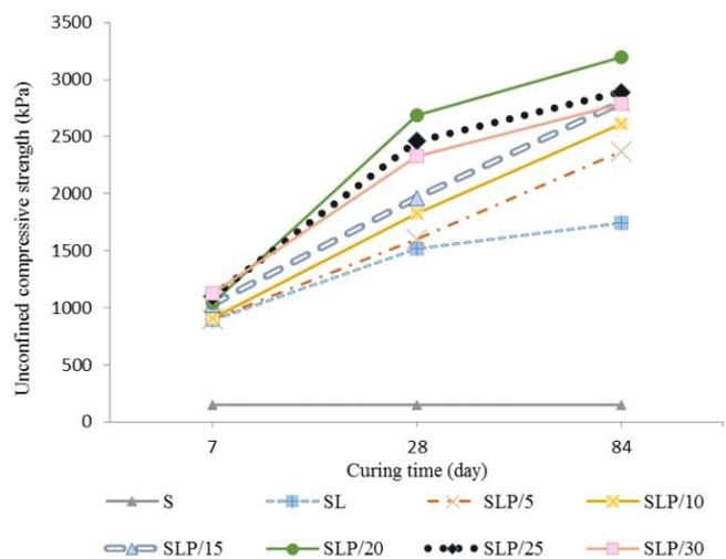
Fig. 9 Unconfined compressive strength of specimens
