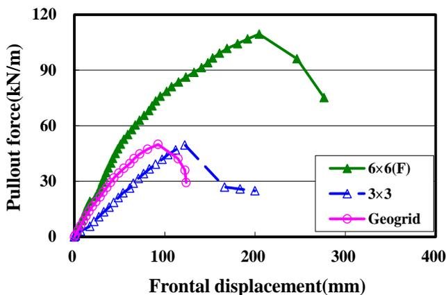
Fig. 13 Comparison between treadmats and geogrid
