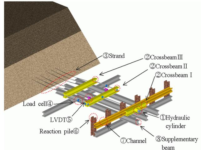
Fig. 2 Schematic of the pullout test apparatus
