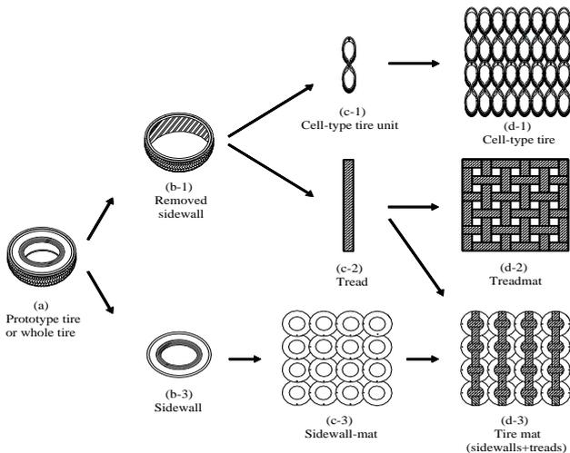
Fig. 1 Combination process to make tire reinforcement materials of four types
