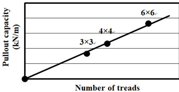
Fig. 12 Pullout capacity of the treadmats with the number of treads
