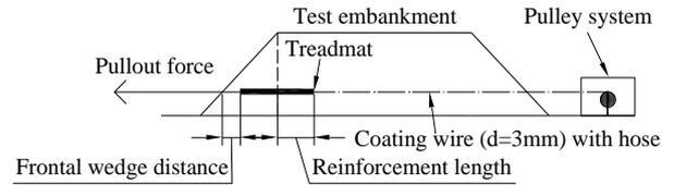
(b) Treadmat half embedded in the embankment
