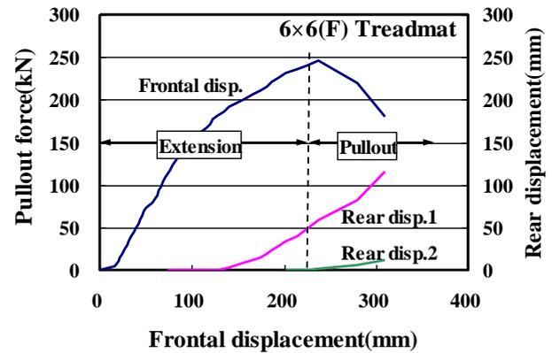
Fig. 8 Typical pullout behavior of the treadmats failed by pullout
