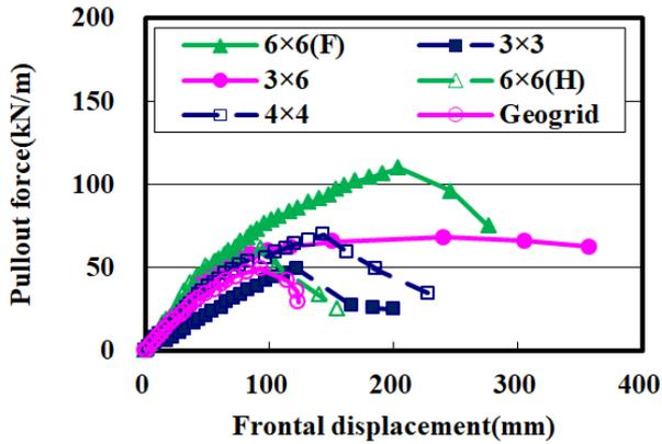
Fig. 11 Pullout behavior of the treadmats with various arrangements
