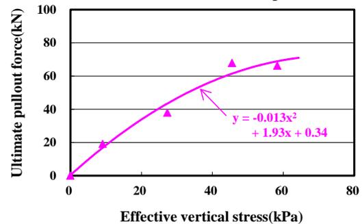
(b) Pullout capacity versus effective vertical stress
