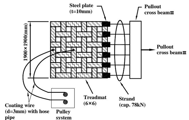
Fig. 3 Plan view of 6×6 treadmat embedded in the embankment
