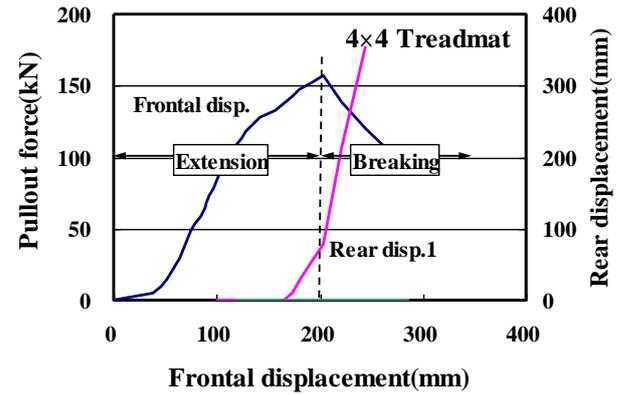
Fig. 9 Pullout behavior of a treadmat failed by breakage
