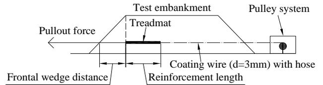
(a) Treadmat fully embedded in the embankment
