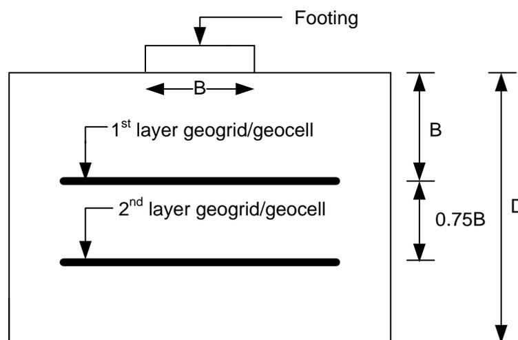
Fig. 3 Typical placement of reinforcement
