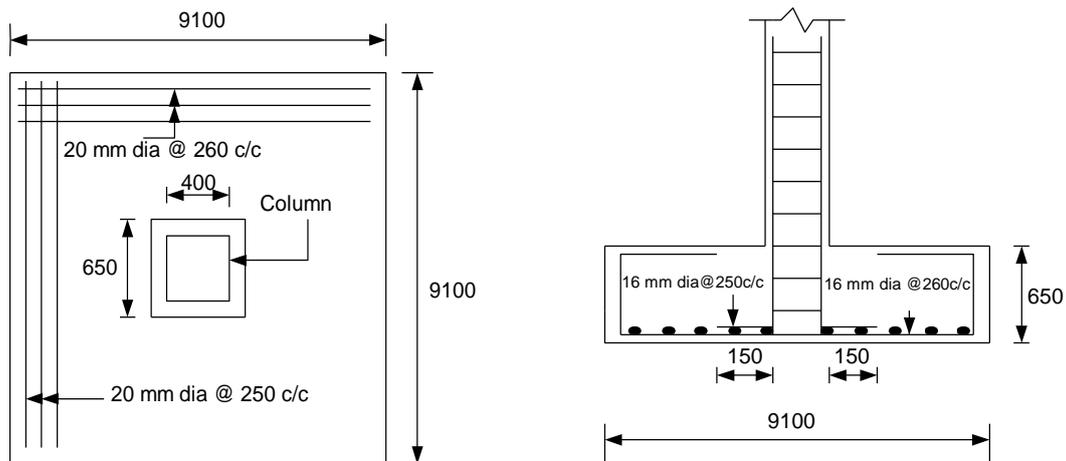
Fig. 8 Placement & Elevation of reinforcement for footing without geocell
