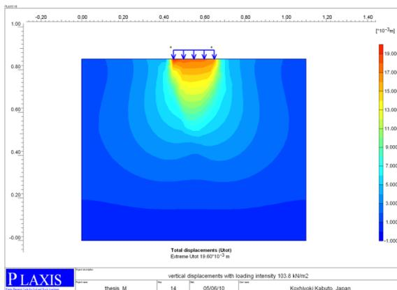
Fig. 6(a) PLAXIS deformation contour for virgin soil
