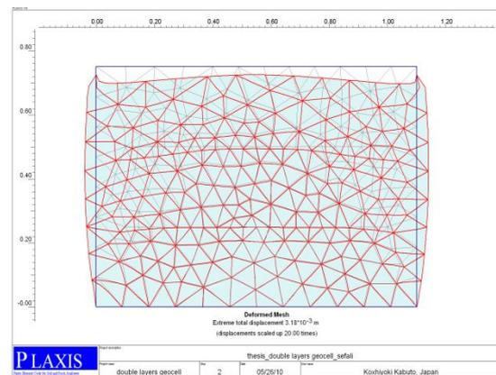
Fig. 6(b) PLAXIS deformation for double layers of geocell
