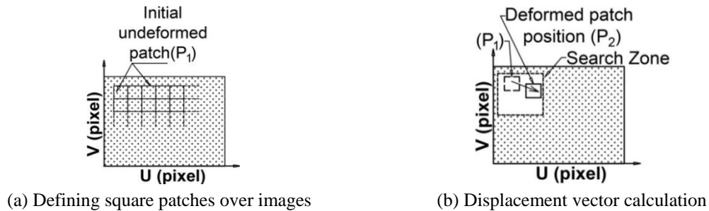
Fig. 2 Determination of displacement vector field
