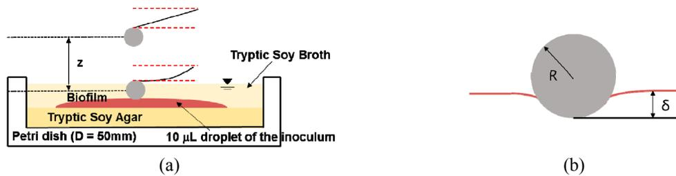
Fig. 2 (a) A schematic diagram of the AFM indentation test on a biofilm sample; and (b) a schematic of an indented surface with a spherical indenter
