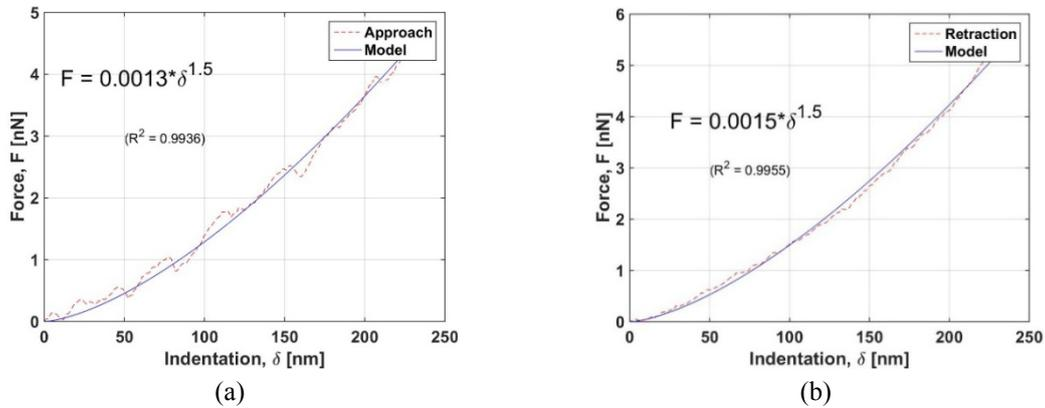
Fig. 5 The force-indentation curves obtained from tests and the model fitting result
