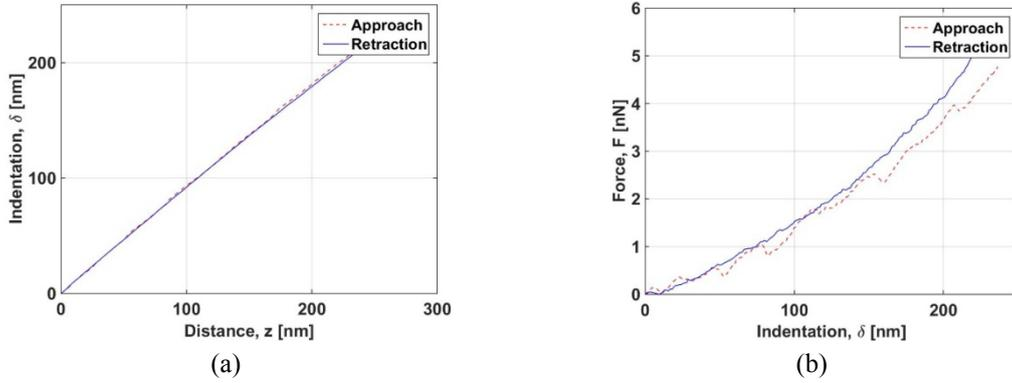
Fig. 4 (a) Indentation-distance relations; and (b) the force-indentation responses during approach and retraction traces
