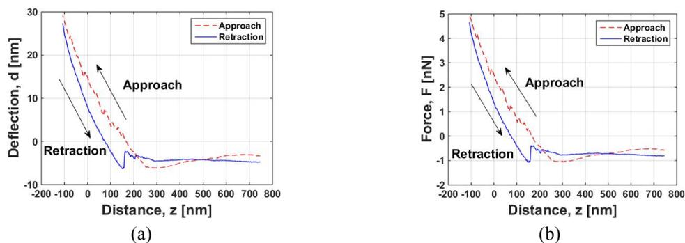
Fig. 3 (a) Deflection-distance responses; and (b) force-distance responses of *S. oneidensis* MR-1 biofilm sample during approach and retraction traces
