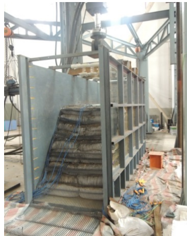
Fig. 1 Test setup & completed embankment: (a) Test setup; (b) photo of the completed embankment before loading
