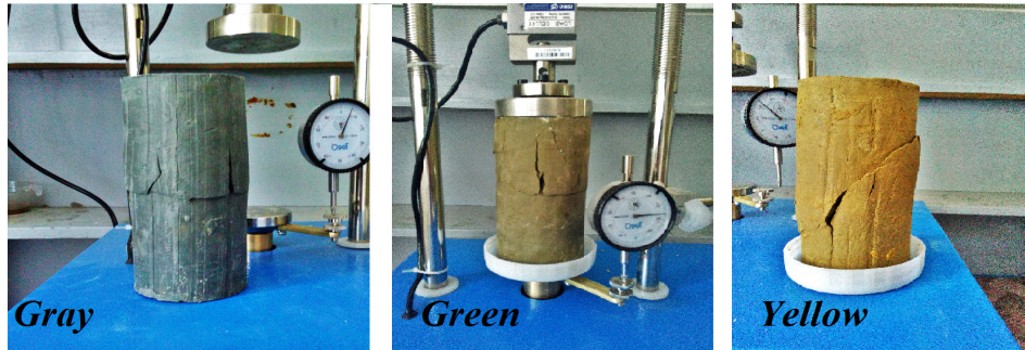
Fig. 8 Three types of marl sample after the UCS tests
