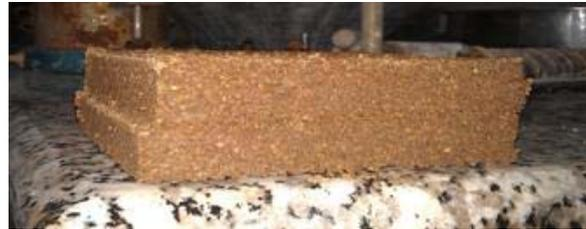
Fig. 7 Sheared sand sample containing 20% bentonite and 10% crude oil contamination
