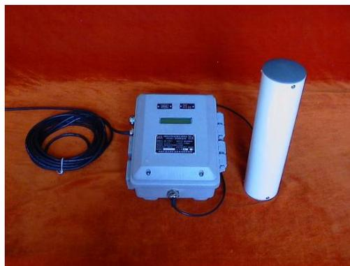
Fig. 6 KBD7 EMR monitor used for measuring the intensity of released stress and the amount of damage pulses
