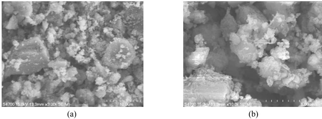
Fig. 10 SEM images of the soil-SSA/lime with 2% nano-SiO<sub>2</sub> additive cured for 56 days: (a) 3,000 $\times$ ; and (b) 10,000 $\times$
