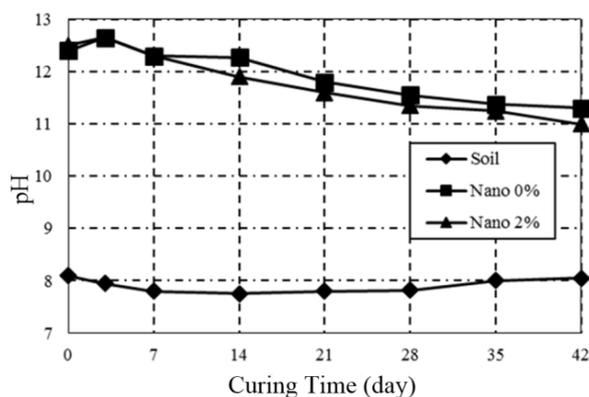
Fig. 4 The relationship between pH and the curing time for the untreated soil, soil-SSA/lime, and soil-SSA/lime with 2% nano-SiO<sub>2</sub> additive
