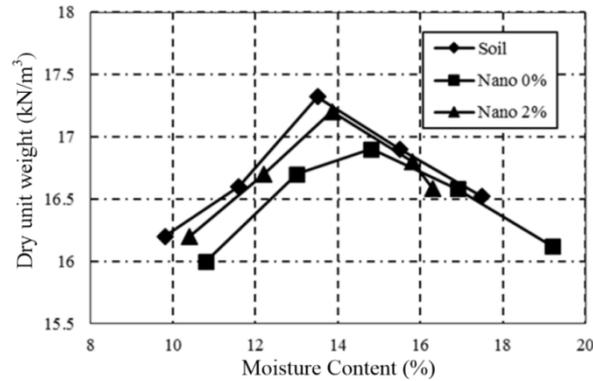
Fig. 2 The results of the OMC and maximum dry unit weight for the untreated soil, soil-SSA/lime, and soil-SSA/lime with 2% nano-SiO<sub>2</sub> additive
