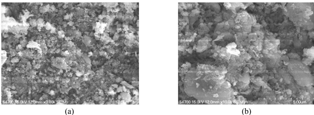
Fig. 9 SEM images of the soil treated with SSA/lime cured for 56 days (a) 3,000 $\times$ ; and (b) 10,000 $\times$
