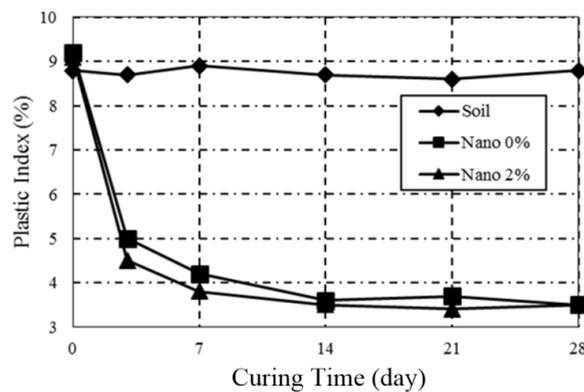
Fig. 3 The relationship between PI and the curing time for the untreated soil, soil-SSA/lime, and soil-SSA/lime with 2% nano-SiO<sub>2</sub> additive
