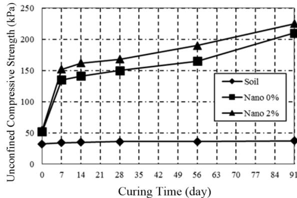
Fig. 5 The relationship between the unconfined compressive strength and the curing time of the untreated soil, soil-SSA/lime, and soil-SSA/lime with 2% nano-SiO<sub>2</sub> additive
