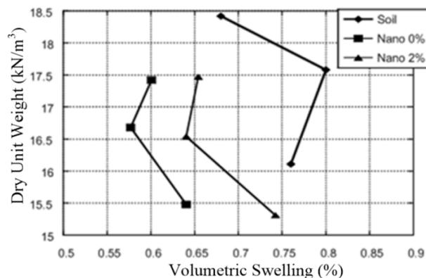
Fig. 7 The volumetric swelling of the untreated soil, soil-SSA/lime, and soil-SSA/lime with 2% nano-SiO<sub>2</sub> additive
