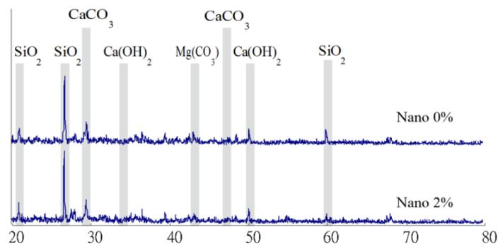
Fig. 11 XRD results of soil-SSA/lime and soil-SSA/lime with 2% nano-SiO<sub>2</sub> additive cured for 56 days
