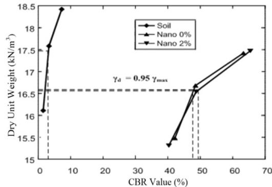
Fig. 8 The relationship between the CBR value and the dry unit weight of the untreated soil, soil-SSA/lime, and soil-SSA/lime with 2% nano-SiO<sub>2</sub> additive
