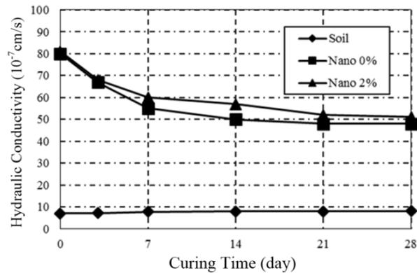
Fig. 6 The relationship between the hydraulic conductivity and the curing time of the untreated soil, soil-SSA/lime, and soil-SSA/lime with 2% nano-SiO<sub>2</sub> additive
