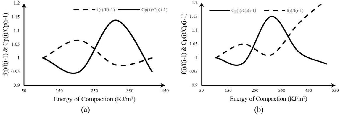
Fig. 4 Average changes in infiltration rate and percent of compaction versus energy of compaction
