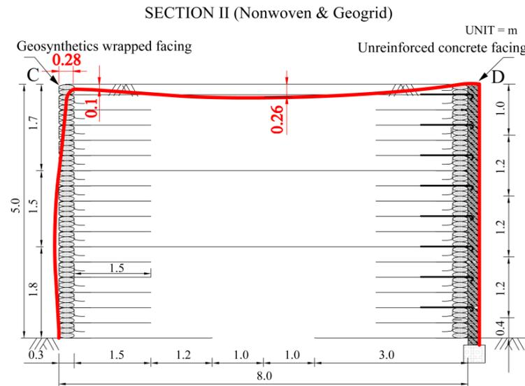
(b) External deformation at SECTION II
