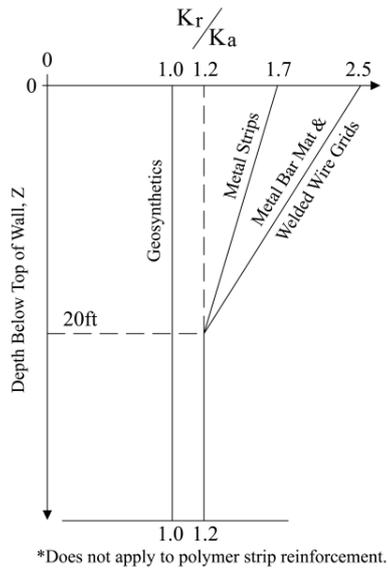
Fig. 6 Variation of the coefficient of lateral stress ratio ( $K_r/K_a$ ) with depth in a mechanically stabilized wall (AASHTO 2002, Elias and Christopher 1997 as cited by Berg *et al.* 2009)
