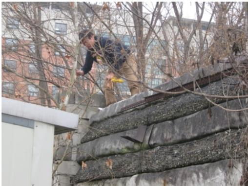
(a) Measurement of horizontal displacements at top
