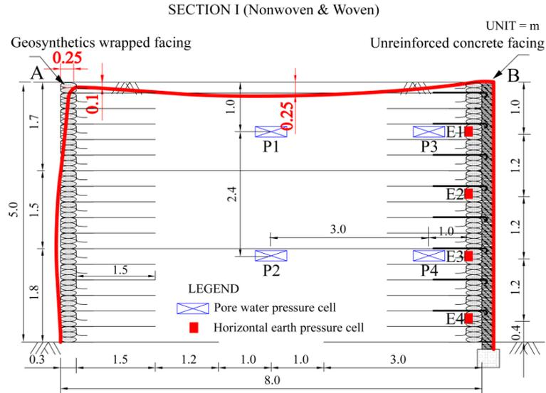
(a) External deformation at SECTION I
