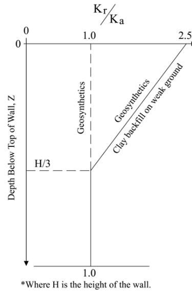
Fig. 7 Variation of the coefficient of lateral stress ratio ( $K_r / K_a$ ) with depth in a GRS wall
