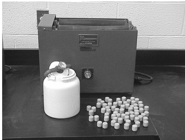
Fig. 4 Jar milling equipment used in the abrasion tests
