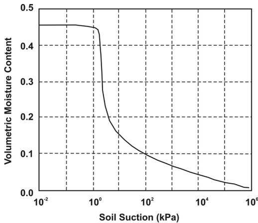
Fig. 8 Soil water characteristic curve
