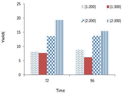
Fig. 2 Effect of reaction time on bioethanol yield at various feed loading
