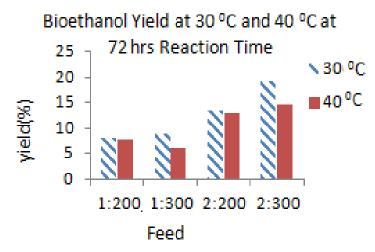
Fig. 1 Effect of temperature on bioethanol yield at various feed ratios
