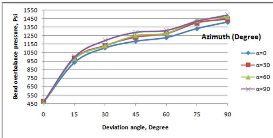
Fig. 9 Minimum overbalance pressure vs. sidetrack orientation in RF stress regime
