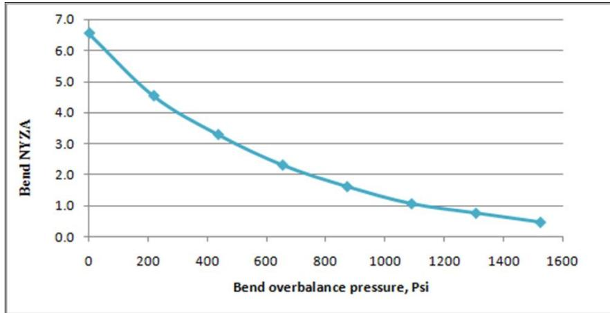
Fig. 2 Variation of NYZA vs. overbalance pressure in bend area for a sidetrack with 45° inclination from the vertical direction and the direction along  $\sigma_h$  in NF-SS stress regime
