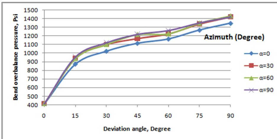
Fig. 10 Minimum overbalance pressure vs. sidetrack orientation in SS-RF stress regime
