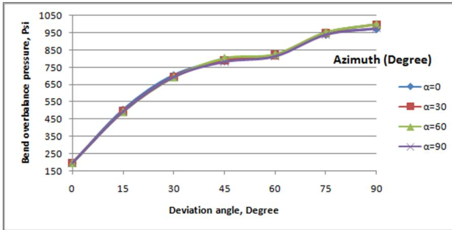
Fig. 6 Minimum overbalance pressure vs. sidetrack orientation in NF with isotropic horizontal stress regime
