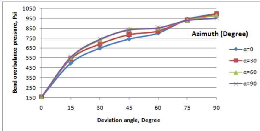
Fig. 5 Minimum overbalance pressure vs. sidetrack orientation in NF stress regime
