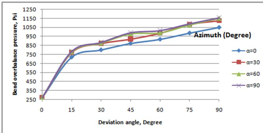
Fig. 7 Minimum overbalance pressure vs. sidetrack orientation in SS stress regime
