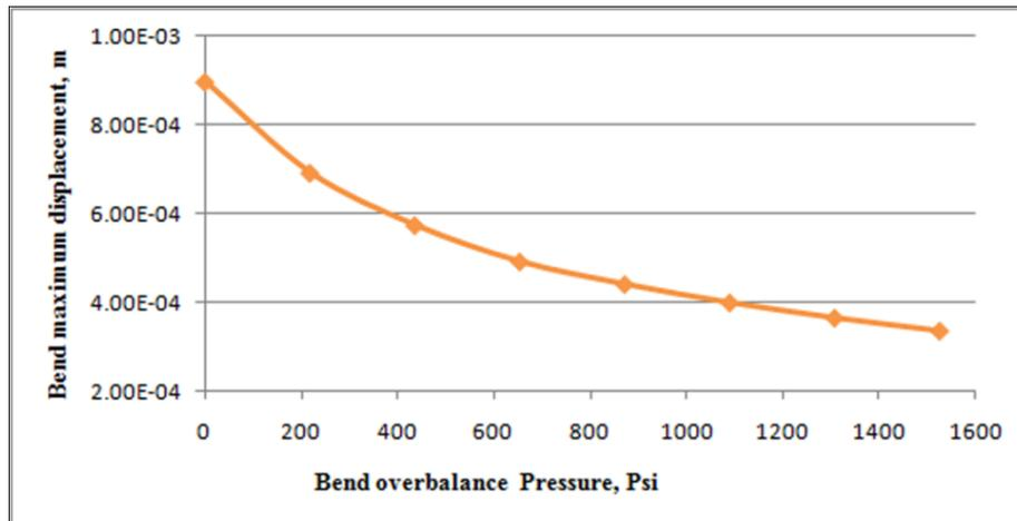
Fig. 3 Variation of displacement vs. overbalance pressure in bend area for a sidetrack with 45° inclination from the vertical direction and the direction along  $\sigma_h$  in NF-SS stress regime
