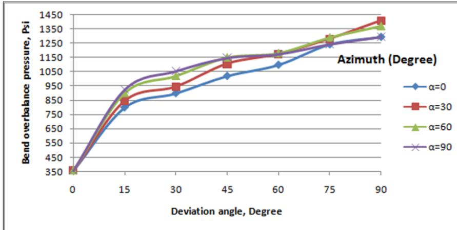
Fig. 8 Minimum overbalance pressure vs. sidetrack orientation in NF-SS stress regime
