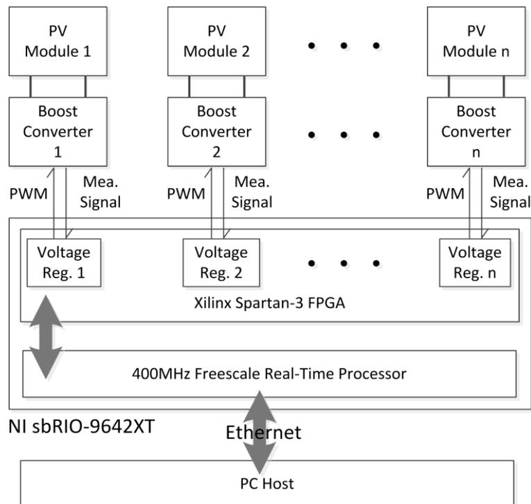
Fig. 3 The control hardware architecture of the novel distributed PV system
