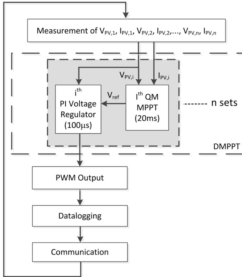
Fig. 4 The DMPPT algorithm for the novel distributed PV system
