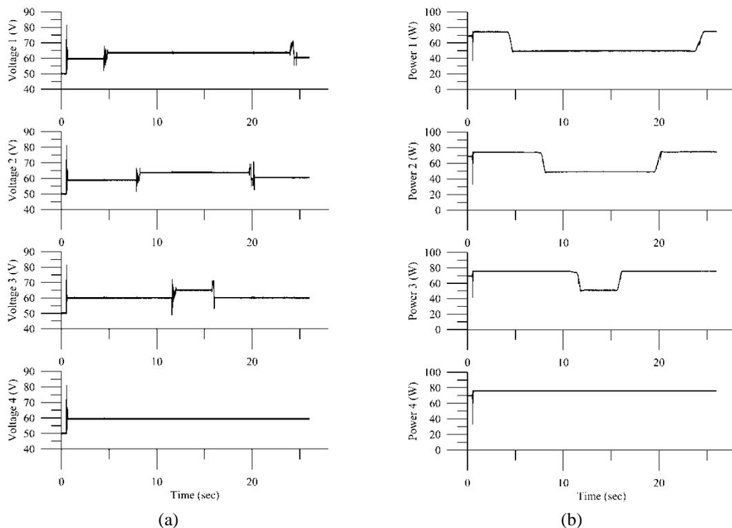
Fig. 8 DMPPT test results from the PV output: (a) voltage and (b) power; panel #1, #2 and #3 were sequentially partial shaded; also note that perturbing a PV panel will not affect other's performance
