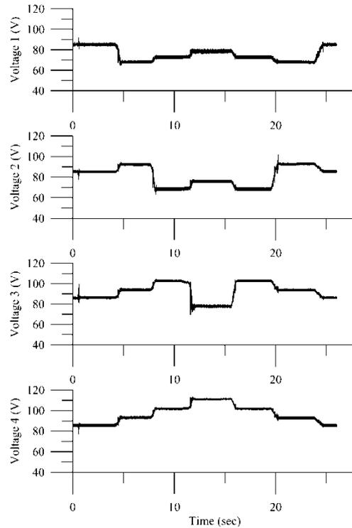
Fig. 9 Voltage measured at MIC output side when panel #1, #2 and #3 were sequentially partially shaded; also note that when a panel was shaded, its output voltage drops whereas others rise in order to keep the panel output power at maximum
