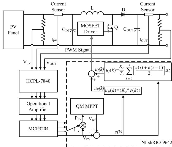
Fig. 7 Schematic design for DC-DC converter, measurement unit, and FPGA operation
