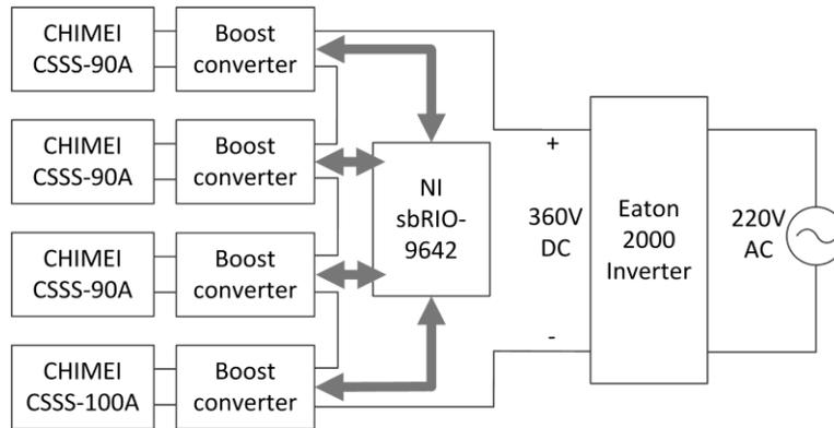
Fig. 6 The distributed PV system design for DMPPT test using 4 PV panels
