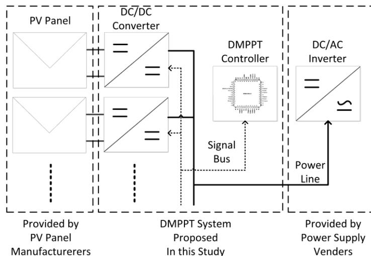
Fig. 2 The proposed distributed PV system using DMPPT controller: FPGA controller for parallel signal measurement, PI voltage regulation; microprocessor for MPPT operation
