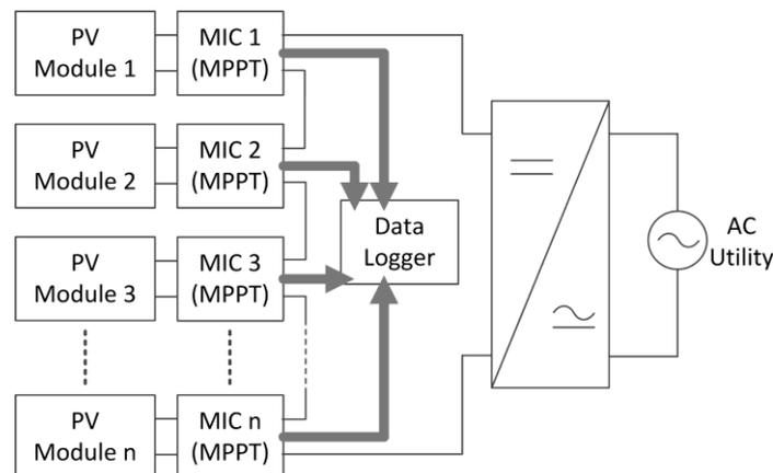
Fig. 1 Block diagram of grid-connected distributed PV system containing serial string panels and module integrated converters
