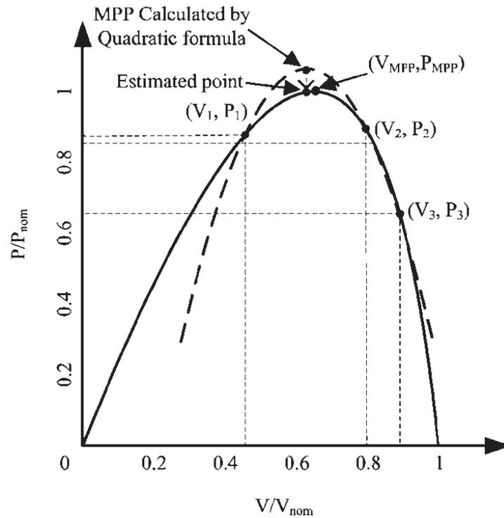
Fig. 5 Illustration of the quadratic maximization MPPT mechanism: solid line—original PV curve; dash line—quadratic approximated PV curve
