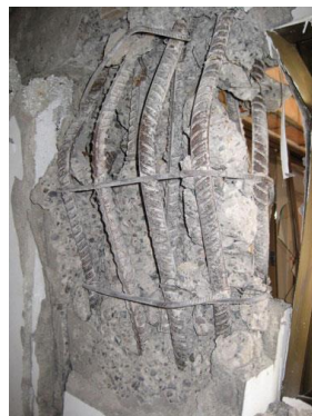
Fig. 3 Buckled reinforcing bars of a reinforced concrete column after Chile earthquake
