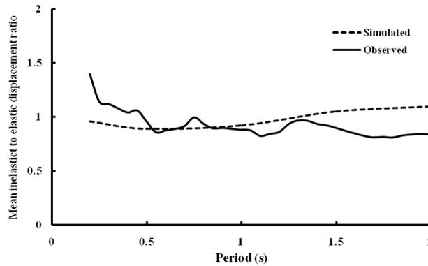
Fig. 5 The mean ratio between inelastic and elastic displacement spectra averaged over all stations. The ratios of inelastic-to-elastic observed spectra computed by the TD method and simulated spectra computed by RV procedure are shown by the solid and dashed lines, respectively
