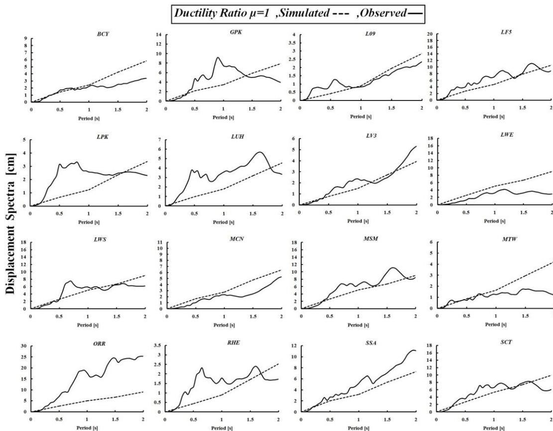
Fig. 3 Recorded and simulated 5%-damped linear displacement spectra (ductility ratio equal to one) at the stations surrounding the fault plane. The station locations are shown in Fig. 2. The observed spectra computed by the TD method and simulated spectra computed by RV procedure are shown by the solid and dashed lines, respectively
