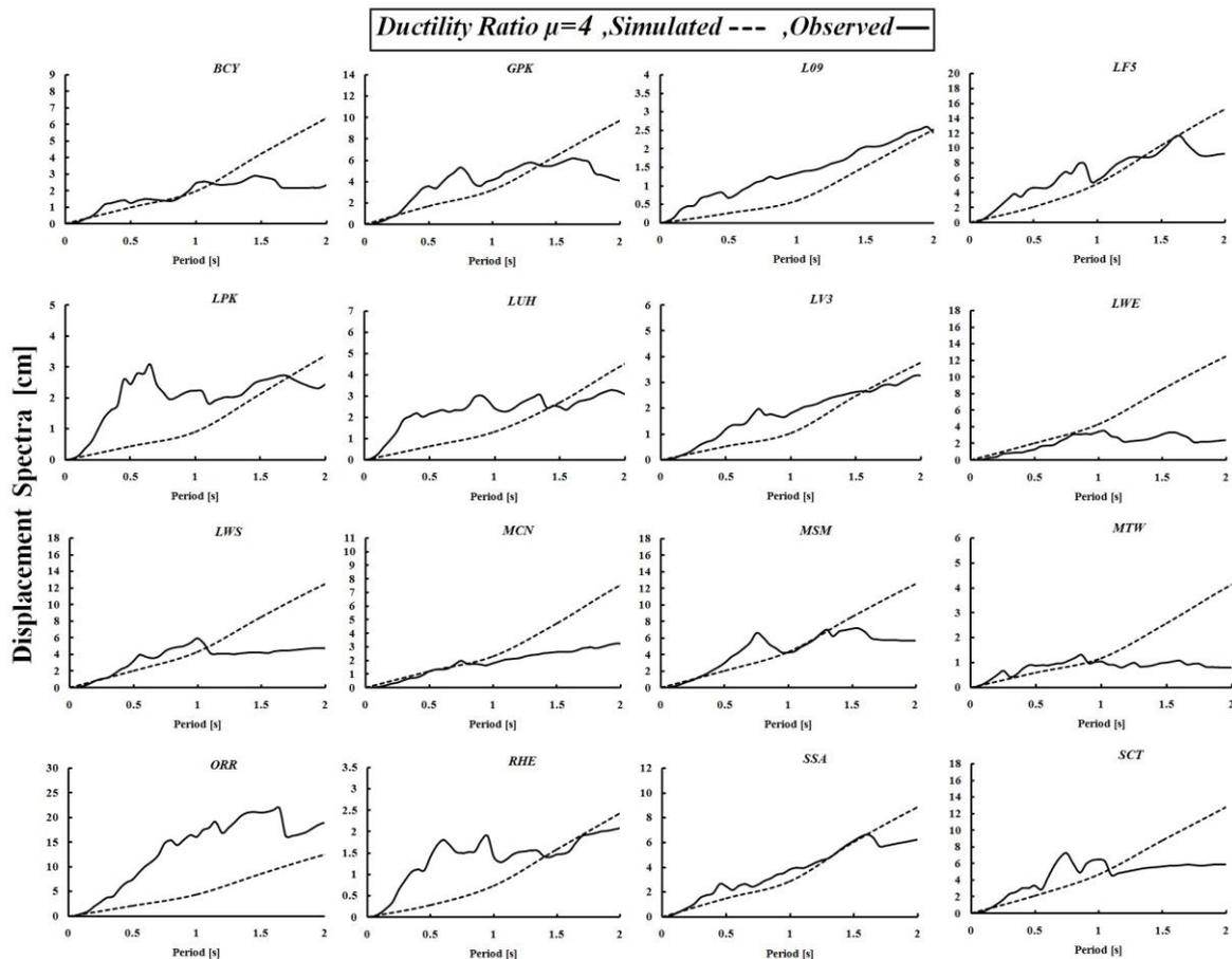
Fig. 4 Recorded and simulated 5%-damped nonlinear displacement spectra (ductility ratio equal to 4) at the stations surrounding the fault plane. The station locations are shown in Fig. 2. The observed spectra computed by the TD method and simulated spectra computed by RV procedure are shown by the solid and dashed lines, respectively
