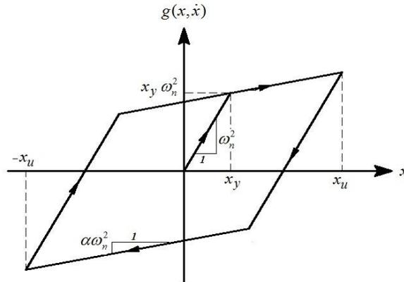
Fig. 1 Bilinear hysteretic restoring force as a function of displacement
