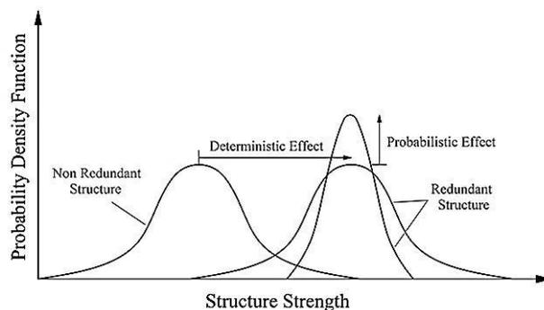
Fig. 6 Effects of redundancy or the overstrength indices  $\Omega_{det}$  and  $\Omega_{pro}$  on structural system strength
