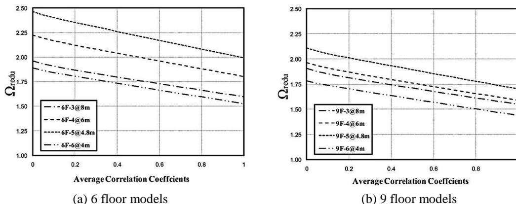
Fig. 9 variation of  $\Omega_{redu}$  versus the average correlation coefficients in 6 and 9 floors models
