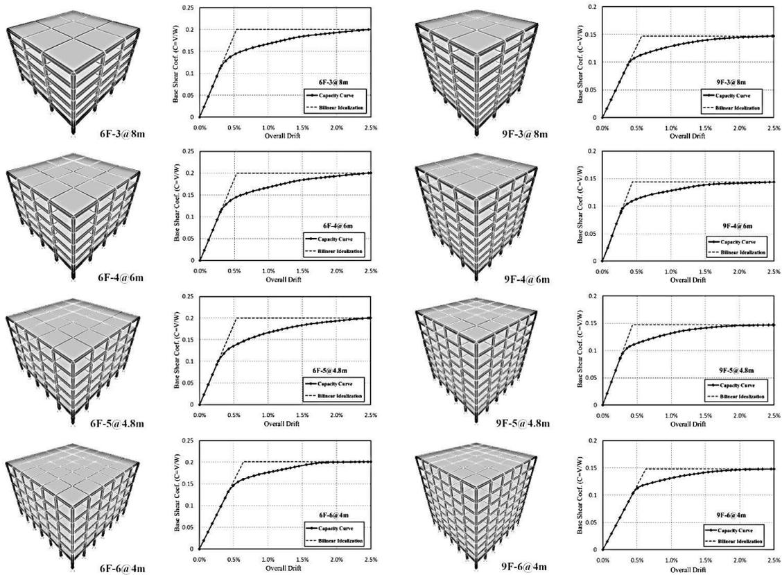
Fig. 7 The capacity curve, bilinear idealization, geometry and reference code of case study models
