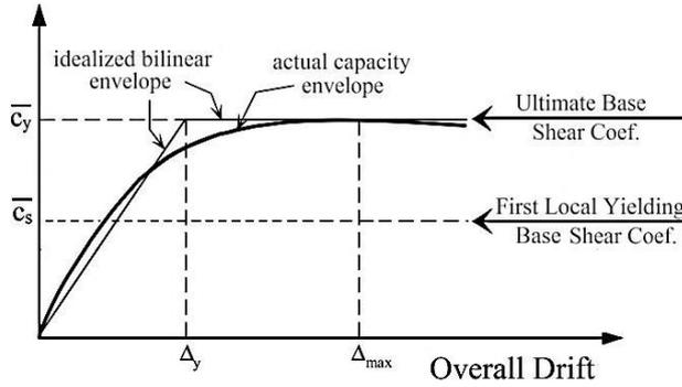
Fig. 2 How to get  $\bar{c}_y$  and  $\bar{c}_s$
