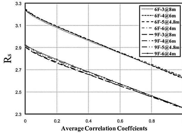
Fig. 10 Variation of total overstrength coefficient versus the average correlation coefficients
