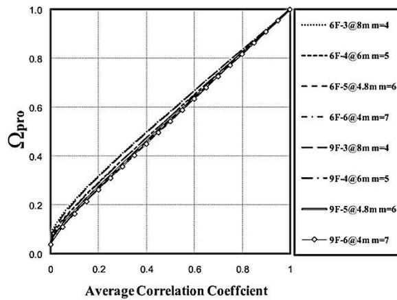
Fig. 8 Variation of  $\Omega_{pro}$  versus the average correlation coefficient and the number of plastic hinge
