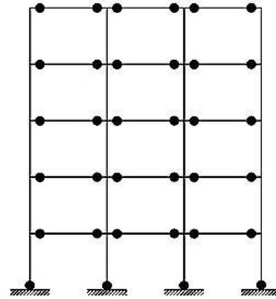
Fig. 3 Sway type failure mode of a general 2D frame
