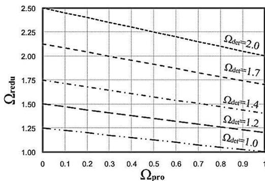
Fig. 5 Variation of  $\Omega_{redu}$  with respect to  $\Omega_{det}$  and  $\Omega_{pro}$  for structural systems with  $kv_e=0.2$
