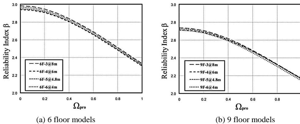
Fig. 12 Variation of the reliability index ( $\beta$ ) of structure with respect to  $\Omega_{det}$  and  $\Omega_{pro}$  for  $\nu_e=0.1$ ,  $\nu=2$
