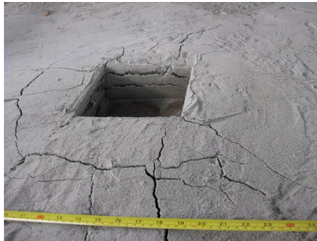
Fig. 7 Punching shear mode of failure in concentric loading test
