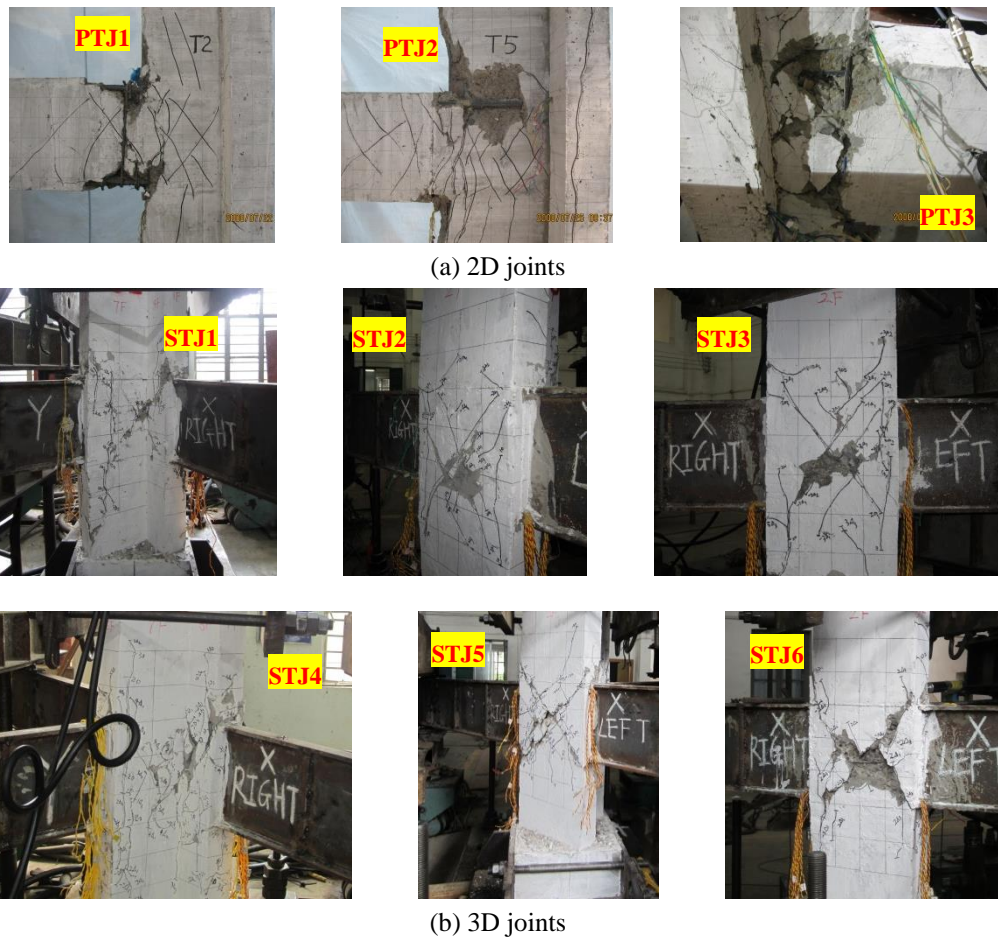
Fig. 6 Failure modes of specimens
