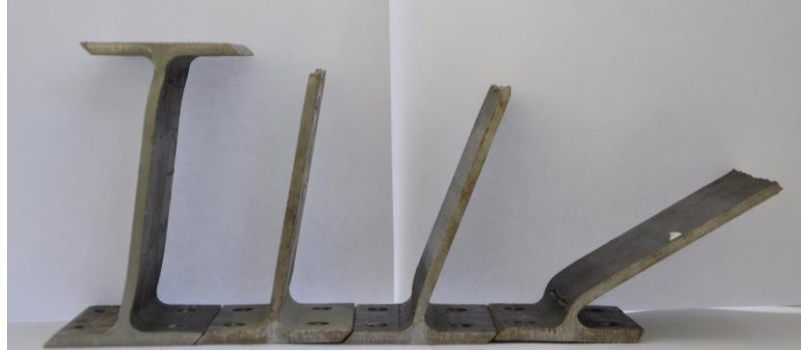
Fig. 19 Close-up views of the deformed web at the maximum drift
